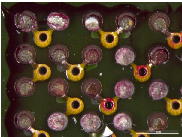
Fig. 24 Image of dye penetrant analysed BGA208 component with the SN100C/SAC305 combination showing the upper left corner of the footprint on the PCB after the component had removed.
