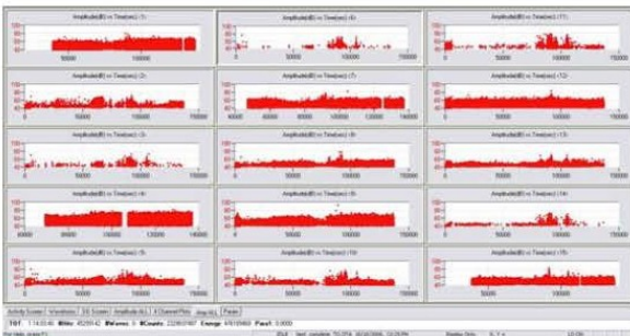
Acoustic Activity in Decibels per Channel for a Transformer Test during a 24 Hour Monitoring Period
