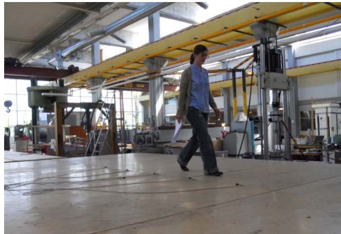
Figure 23. Measurement setup for the walking subtest.
