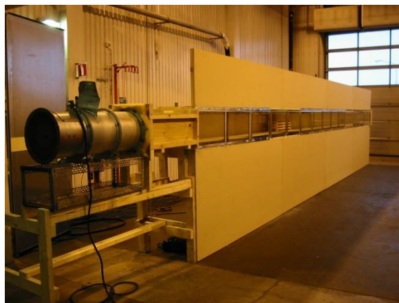
Figure A1 A photo of a model-scale tunnel used by Ingason [28-29] for tests with longitudinal ventilation.
