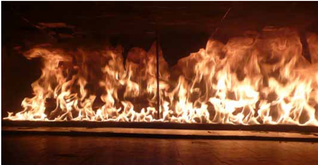
Figure 5.8 Flames inside the model building during Test 1.
