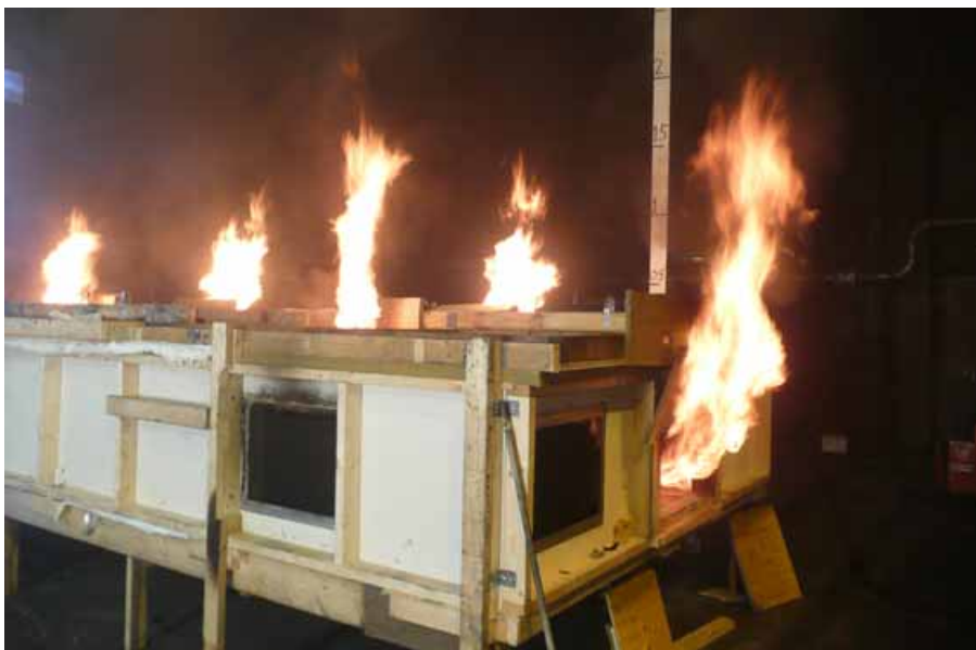
Figure 5.7 Flames out through openings during Test 2.
