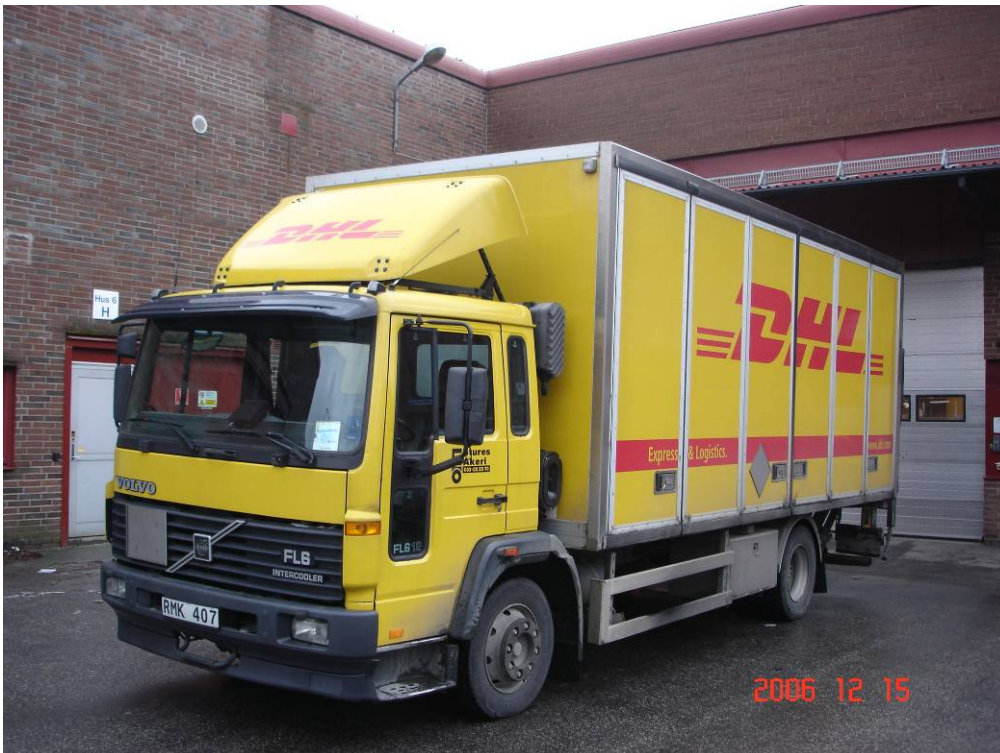
A freight truck with a box with solid walls and ceiling, typically used in the Nordic countries.
