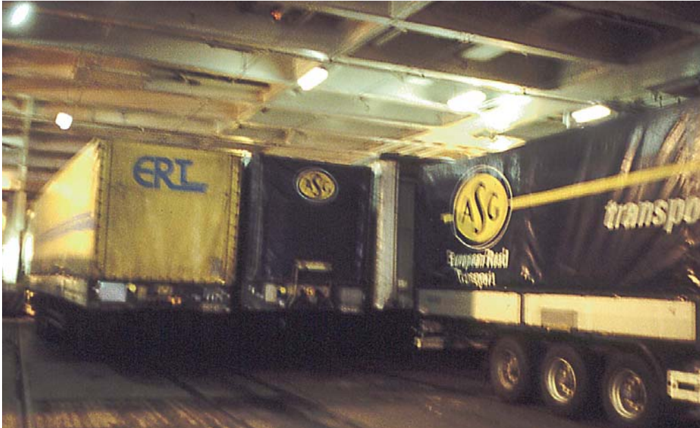
Freight trucks on a ro-ro deck, illustrating the short distance between the vehicles and the limited deck height.
