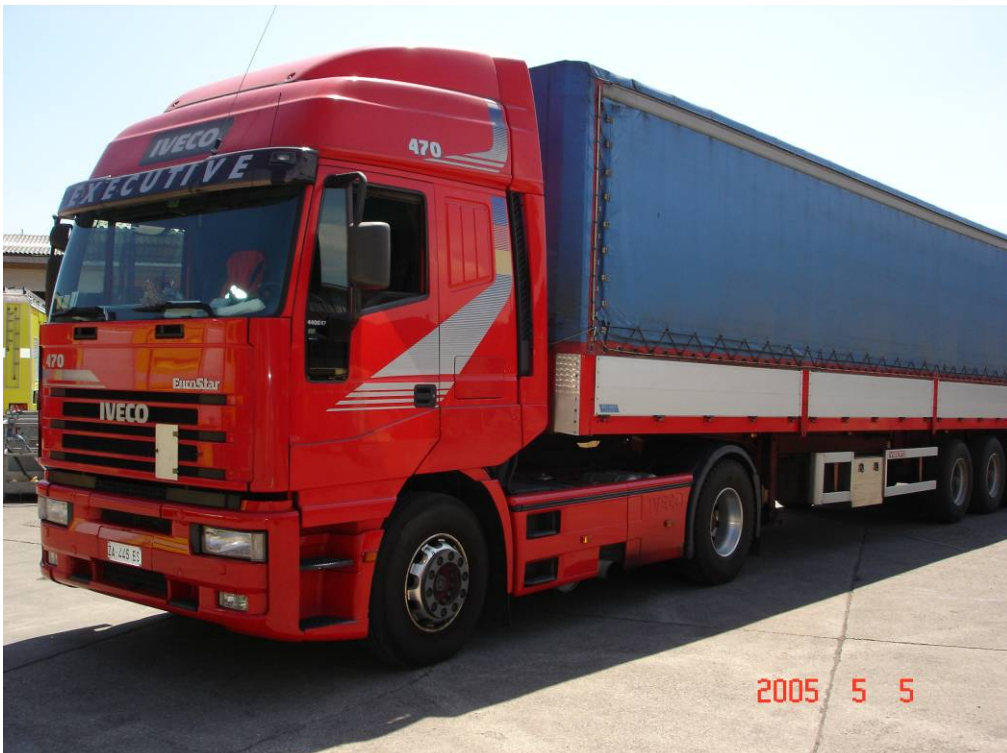
A common type freight truck used throughout Europe, where the trailer is covered by a tarpaulin, both on the sides (“curtain sides”) and over the ceiling.
