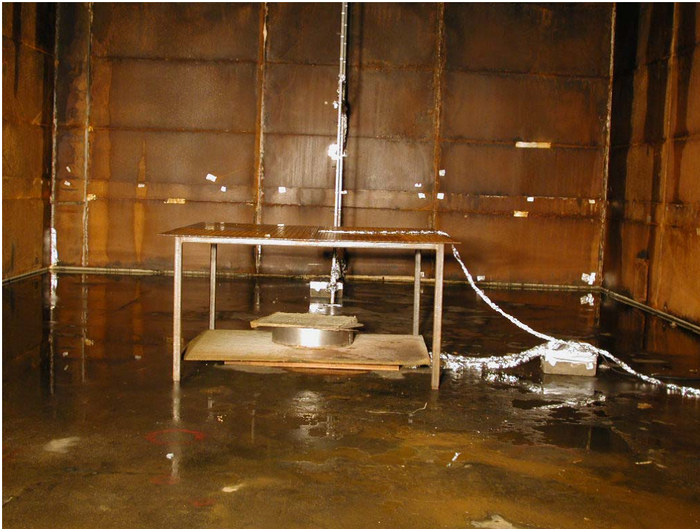
Photo B5 The horizontal obstruction steel plate, with the fire tray positioned on a load cell.
