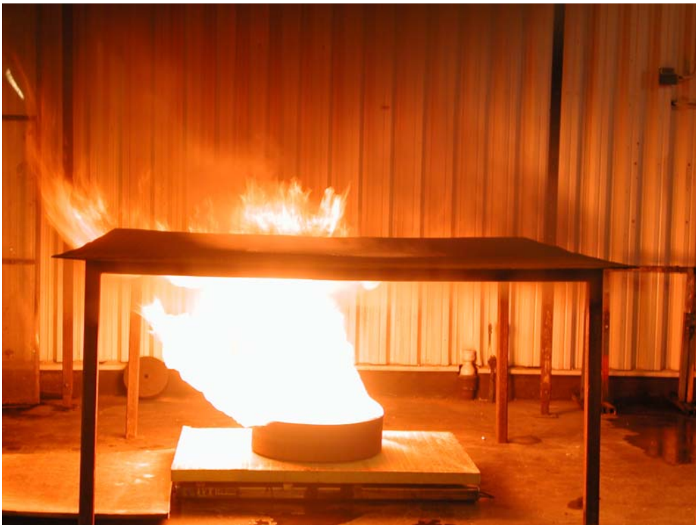
Photo B6 The size of the obstructed 500 kW heptane pool fire.
