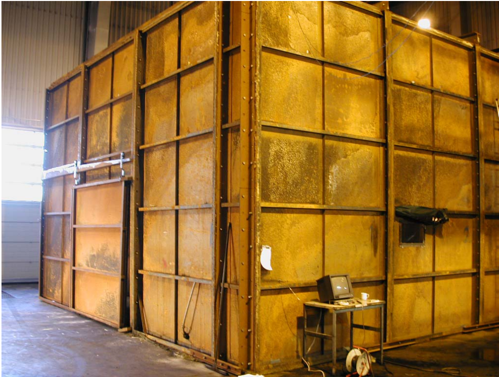
Photo B1 The 500 m 3 test compartment.
