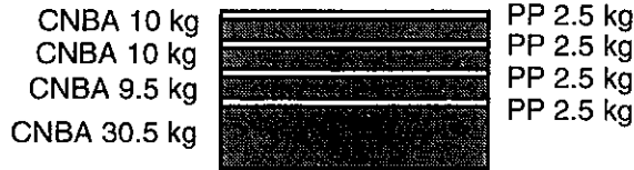
Figure 12.1 In the test CNBA2 non-woven polypropylene was added to the CNBA, distributed in separate layers with polypropylene on top.
