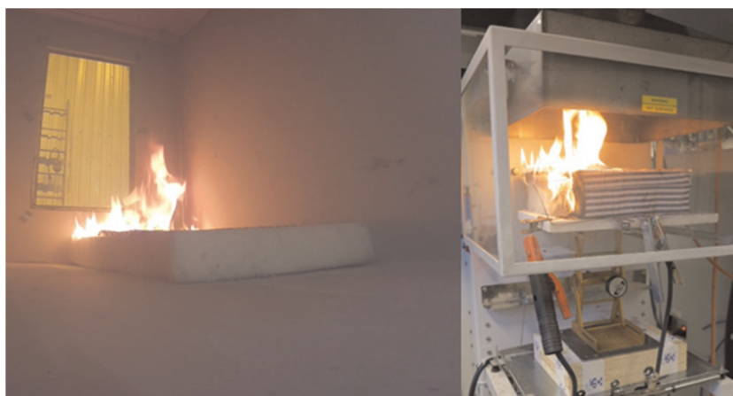
Fig. 7. Mattress fire source in the sleeping compartment mockup (left) and in the calorimeter setup (right).
