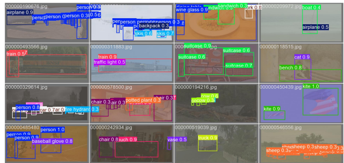
Fig. 1. 6 color transformations and 32 YOLO model variants are evaluated for establishing \Delta E thresholds. An excerpt of results of YOLO11x on images transformed with “Pull Mean” at \Delta E = 21 is shown above.
