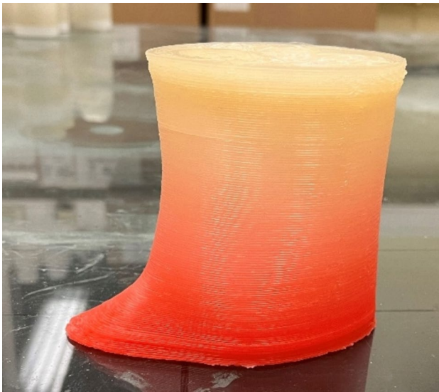
Fig. 9 3D shaped demonstrator created by mixing two polymer granulates, #309 with red additive and #310 color-less. The relative portion of the red decreases gradually from the bottom to the top
