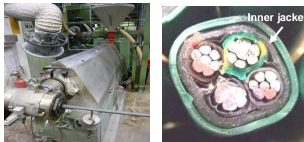
Fig. 8: Extrusion of cable with inner jacket of recyclate compound XLPE/LLDPE (20/80)
