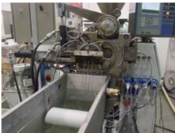
Fig. 5: Extrusion screening PVC compound
