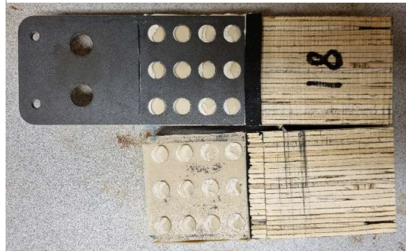
Figure 11: Failure solely in the glue dowels and in the steel-to-wood interface.
