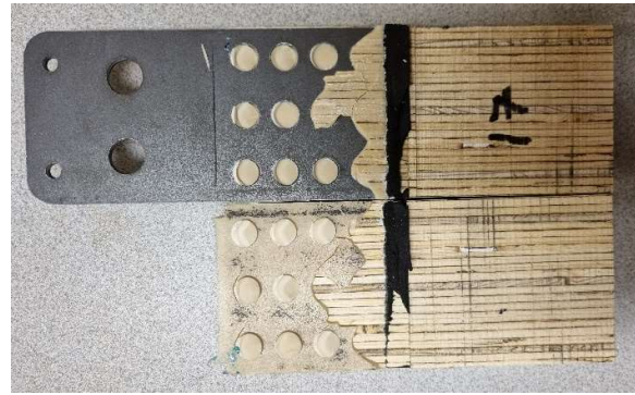
Figure 10: Combined failure in the glue dowels, the steel-to-glue interface and in the wood-to-glue interface.
