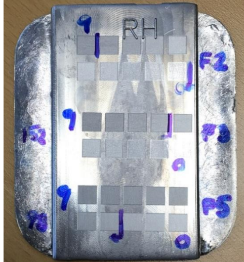
Figure 1. A HPDC test plate with various laser treatments. The backside of this palate was not treated by the laser. The size of the plate is about 60x70mm.
