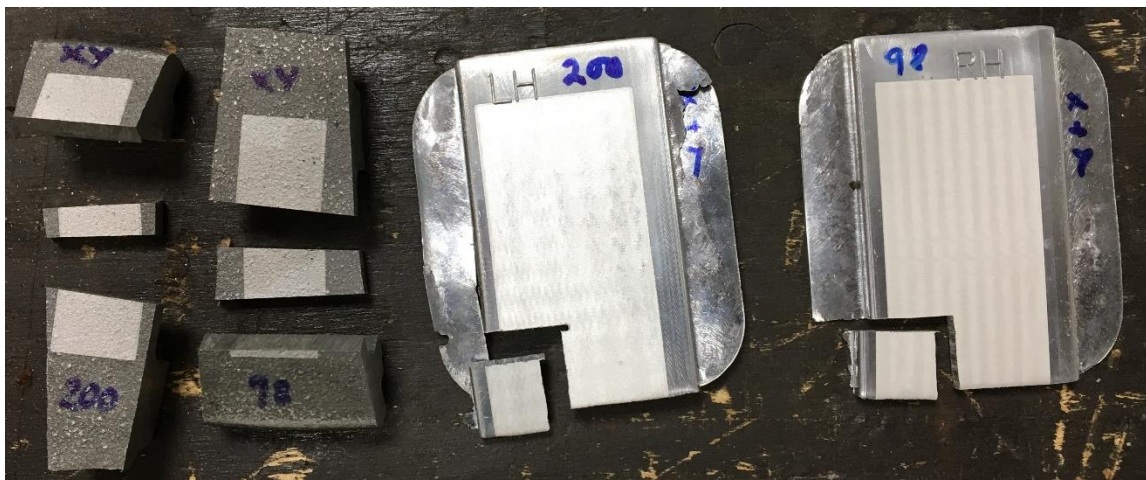
Figure 7. Cuts made before mounting and preparation for examination in light optical microscope.
