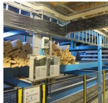
A project for weighing sawn timber packages started in April 2013. The aim of the demonstration is to improve accuracy in hitting the target moisture content in sawn timber by weighing the wood packages before drying. The package weight is used to optimize the drying program based on the ingoing material of each batch.
