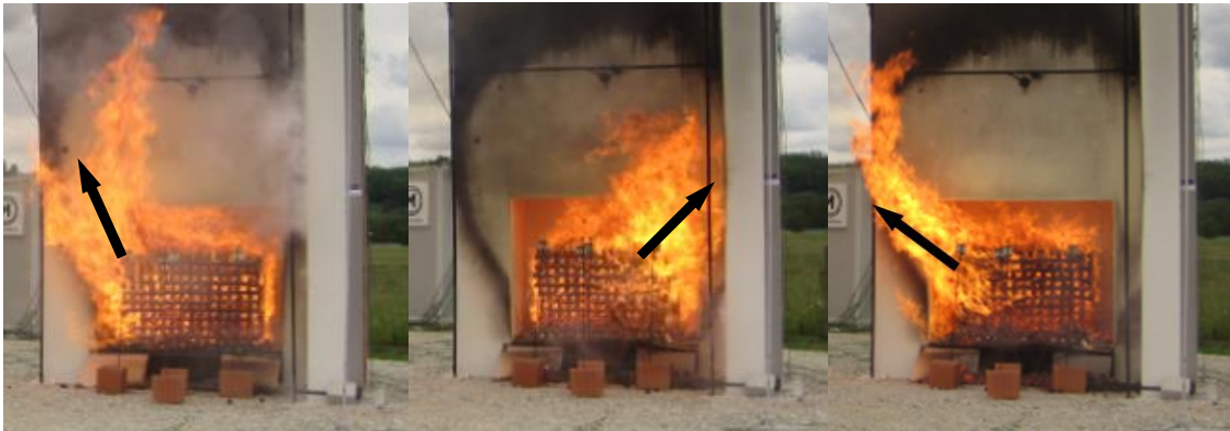
Figure 9: Changing directions of the fire plume during an outdoor BS 8414 façade fire test ( Test 2 , Anderson et al. 2017)
