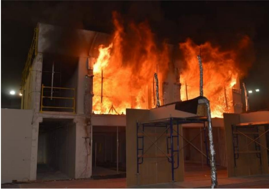
Figure 1: Compartment fire test after flashover (Hasburgh et al., 2018)
