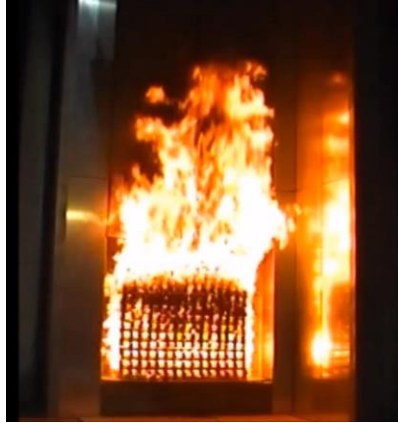
Figure 8: Typical fire plume during an indoor BS 8414 façade fire test.
