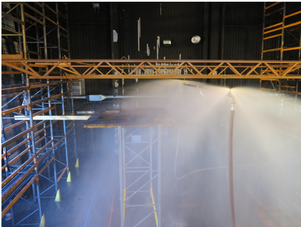
Figure 8 Test 2.6: The water spray pattern of the Tyco model EC-14 sprinkler at a pressure of 3.2 bar and a spacing of 5.0 m. The water flow rate per sprinkler was 354 liter/min.
