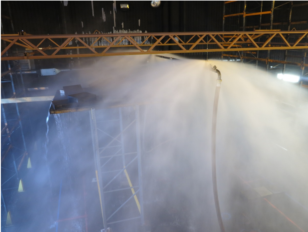
Figure 9 Test 2.1: The water spray pattern of the Tyco model EC-14 sprinkler at the maximum pressure of 6.8 bar obtained with the pump. The water flow rate per sprinkler was 520 liter/min.
