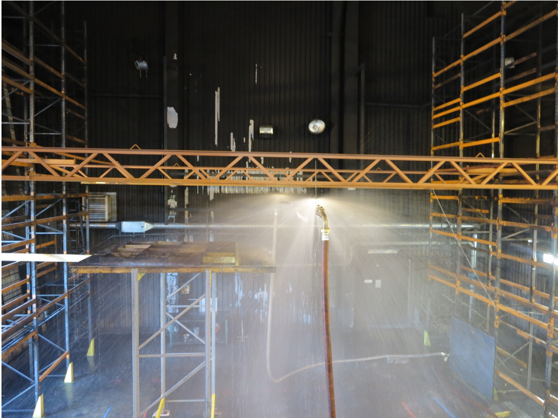
Figure 10 Test 2.8: The water spray pattern of the modified Tyco model EC-25 sprinkler at a pressure of 0.95 bar and a spacing of 4.2 m. The water flow rate per sprinkler was 354 liter/min. The modification of the sprinkler deflector provided improved coverage on the top of the platform but a reduced discharge density on the floor.
