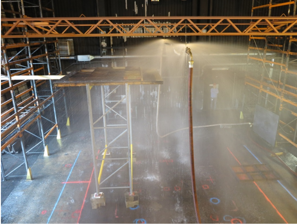
Figure 11 Test 2.13: The water spray pattern of the combined non-modified Tyco model EC-25 (the furthest sprinkler) and Tyco model EC-14 sprinkler at a pressure of 1.7 bar and a spacing of 4.2 m. The total water flow rate was 708 liter/min.
