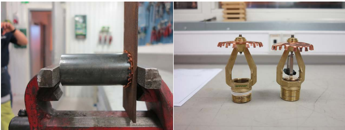
Figure 3 The modification of the deflector of the Tyco model EC-25 sprinkler (left) and the result (right). The modified sprinkler is shown to the left.
