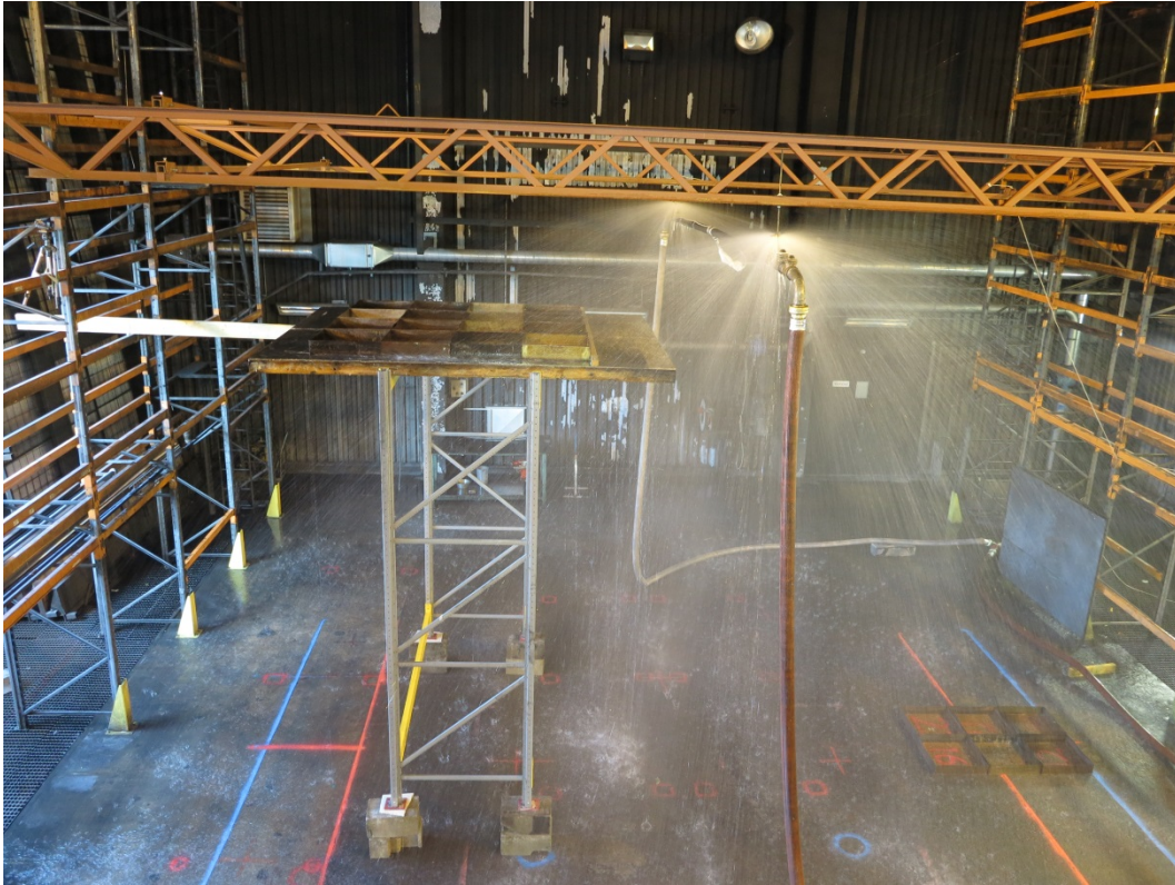
Figure 1 The test set-up, with the platform that simulated the freight truck trailer and the sprinkler pipe positioned at the centerline of an imaginary tunnel. The water distribution was measured with trays positioned at the top of the platform as well as on the floor. Imaginary sidewalks and the outer boundary of the tunnel are drawn on the floor.
