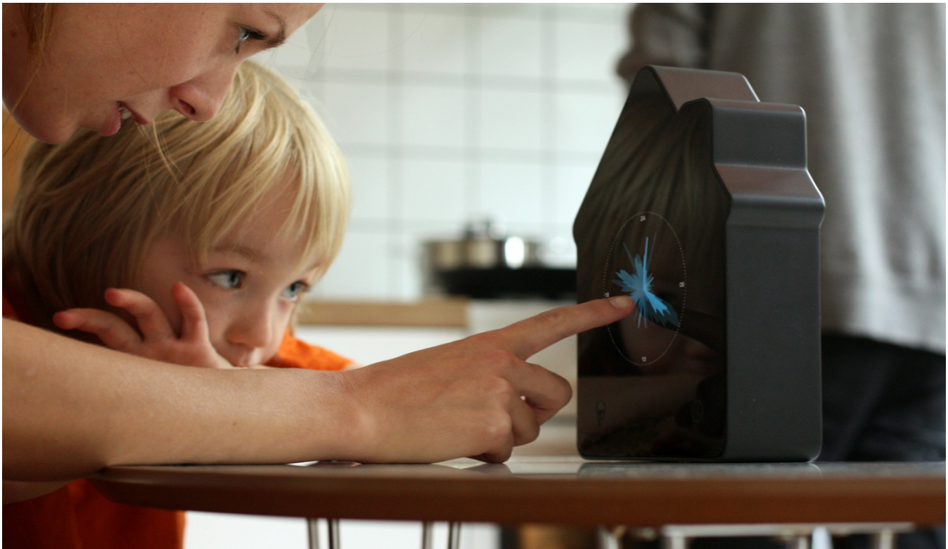
Figure 4: The Energy AWARE Clock in the 24 hour view, showing the electricity consumption for the whole day and two days back in time.
