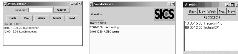
Figure 5: Three user interfaces to the calendar service generated from the same interaction acts. The two to the left are generated by the Java Swing interaction engine using two different customization forms. The one to the right is generated by the Tcl/Tk interaction engine.
