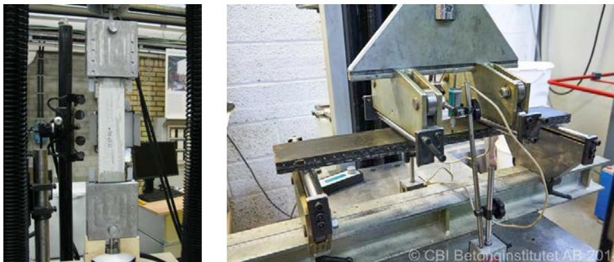
Figure 3: Setup for tensile (upper left) and flexural strength testing (upper right).
