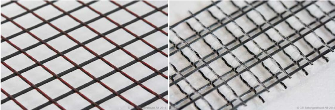
Figure 2: Types of carbon textile fibre reinforcement: 2d grid (left) and 3d grid (right).
