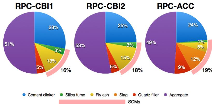
Figure 6: Comparison of clinker replacement levels (on the solid content) by supplementary cementitious materials (SCMs) for the RPC mix approaches of CBI and ACCIONA.
