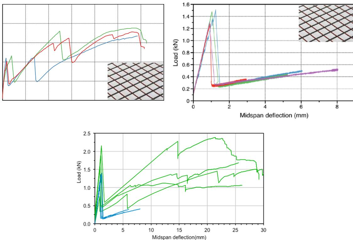
Figure 5: Results from tensile (upper left) and flexural (upper right) tests with mix RPC-CBI1 with 2d carbon textile fibre reinforcement. Lower graph: Results flexural tests with mix RPC-CBI1 with 2d carbon textile grids and additional carbon fibres. Blue: textile grid only, green: textile grid and carbon fibres.
