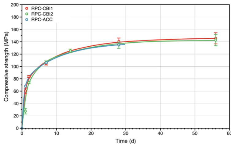
Figure 4: Development of compressive strength for the three different mixes.
