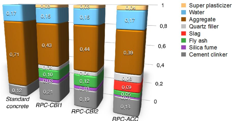
Figure 1: Composition of the RPC mix formulations compared to a standard concrete (in volu fractions).
