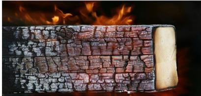
**Figure 1.** The char layer provides an effective heat insulation to maintain the load-bearing resistance. However, heated timber exhibits less strength which has to be considered in calculation models [Image source: *Fire Safety In Timber Buildings*].
