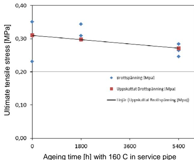
Figure 14: Regression curve for ultimate tensile stress obtained from pulling method.
