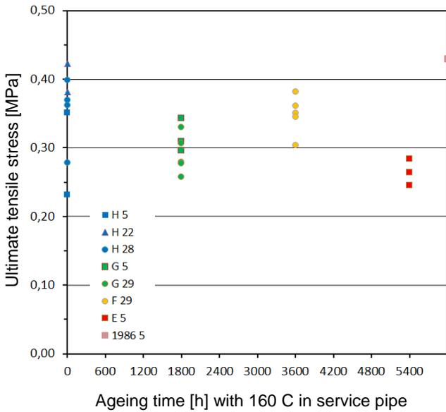
Figure 9: Measured ultimate tensile stress of test specimens as function of ageing time in laboratory and also for a pipe GA which have been in service for 25 years. Length of specimen is part of notation.
