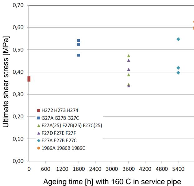
Figure 10: Measured ultimate shear stress of test specimens as function of ageing time in laboratory and also for pipe GA which have been in service for 25 years. For 3600 h, results for specimens of both length 25 mm and 5 mm are given.
