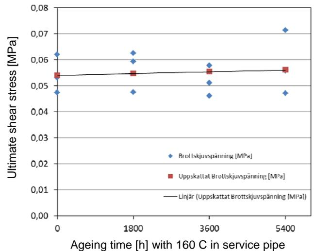
Figure 13: Regression curve for ultimate shear stress obtained from turning method.
