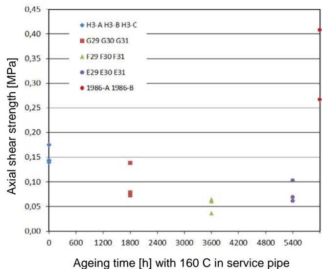
Figure 7: Axial shear strength of accelerated aged district heating pipes and a pipe GA which have been in service in 25 years.
