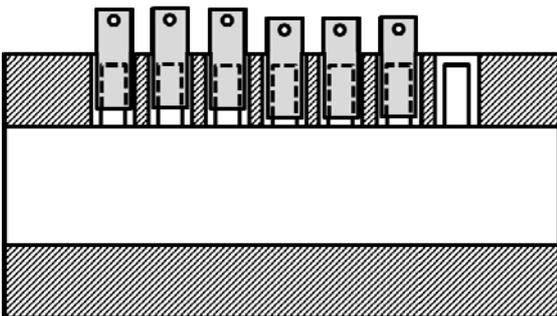
Figure 4: District heating pipe with cylindrical test specimens on to which aluminium pipes holders have been fixed by use of glue.
