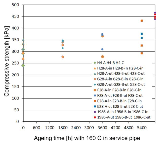
Figure 8: Compressive strength of accelerated aged district heating pipes and a pipe GA which have been in service in 25 years.
