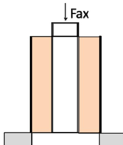
Figure 1: Sketch of axial shear strength test.
