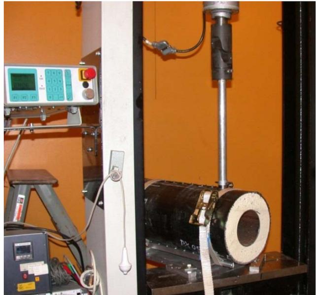
Figure 5: Picture of laboratory equipment for pulling cylindrical specimens loose.
