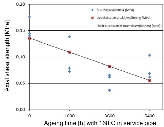
Figure 12: Regression curve for axial shear strength.
