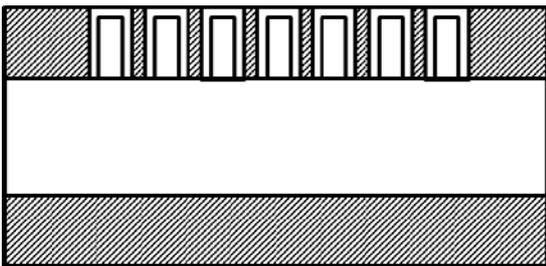
Figure 3: District heating pipe with uncovered cylindrical test specimens still attached to the service pipe.
