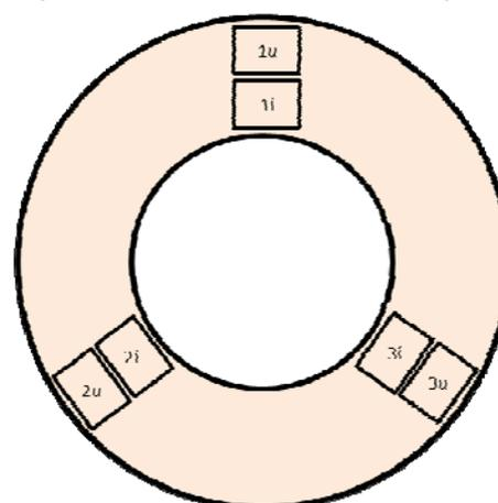
Figure 2: Sketch of positions of test specimens for compressive strength.
