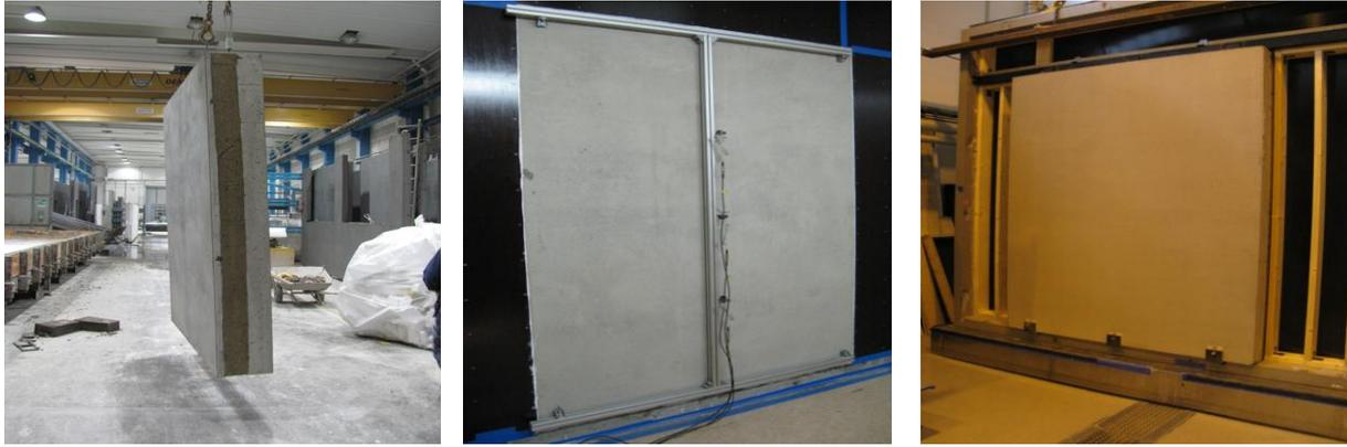
Figure 4 – Sandwich element (left), mounting for the wind load testing (middle and left).
