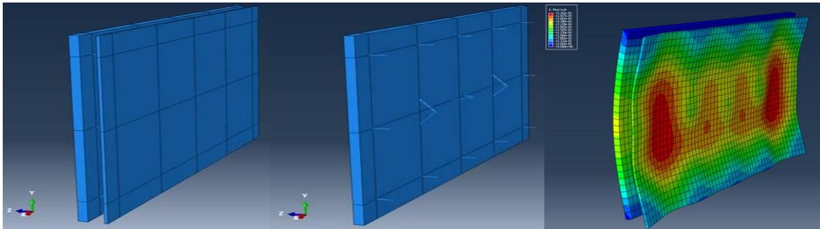
Figure 1 - FE-model of a sandwich element (left, middle) and the total deformation  $U$  for dimensioned wind  $W = 1.57 \text{ kN/m}^2$ .
