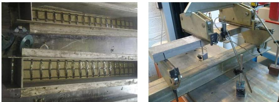
Figure 2 – Casting of the beams (left) and set up for bending strength measurement (right).
