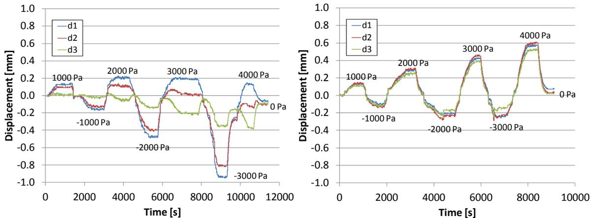
Figure 5 - Displacement vs. time for the respective gauges for carbon fibre reinforced element (left) and glass rod reinforced element (right).
