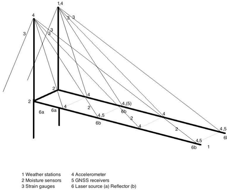
**Figure 1** – Schematic picture of location of the sensors (not drawn to scale). The sensors depicted on the deck will be mounted beneath the bridge deck.
