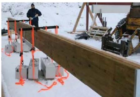
Figure 7. Modulus of elasticity.
