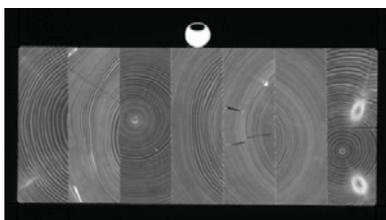
Figure 8. CT image of a cross-section of a beam. On top of the beam is a jar containing water as a density reference.
