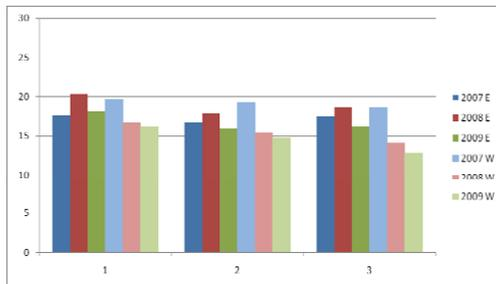
Figure 12. Moisture content of one beam B3 measured at end positions (east and west), positions 1-3 according to figure 6.
