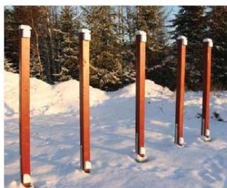
Figure 5. Columns with top surface covered with a sheet metal.
