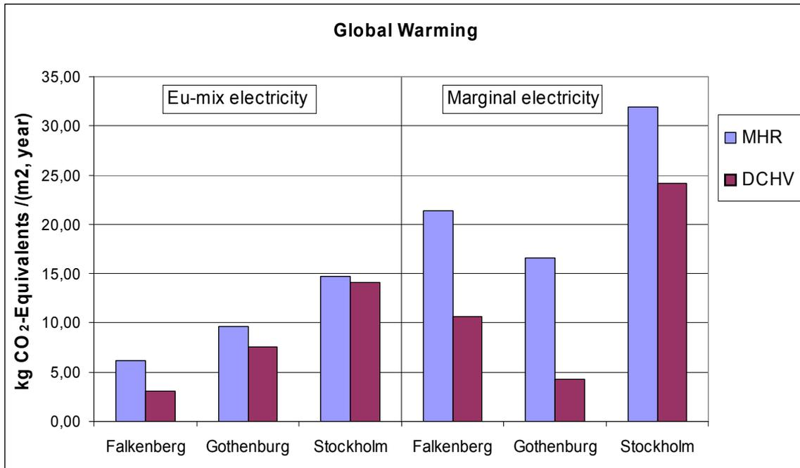
**Figure 3. Impact of global warming for MHR and DCHV ventilation principles in the Tånga school, sited in three different cities. Electricity is considered as an EU mix to the left and as marginal production (peak power) to the right.**
