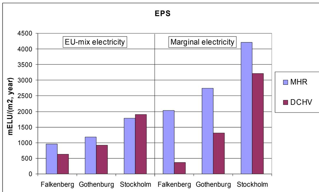
**Figure 4. Environmental assessment with the EPS method for MHR and DCHV ventilation principles in the Tånga school, sited in three different cities. Electricity is considered as an EU mix to the left and as marginal production (peak power) to the right.**
