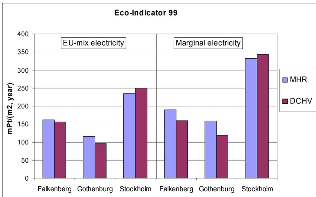
**Figure 5. Environmental assessment with the Eco-Indicator 99 method for MHR and DCHV ventilation principles in the Tånga school, sited in three different cities. Electricity is considered as an EU mix to the left and as marginal production (peak power) to the right.**
