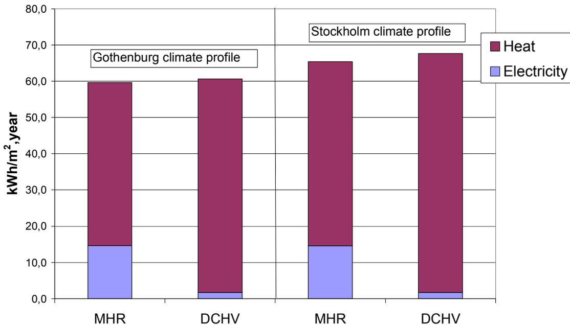
**Figure 2. Electricity and district heating use for two ventilation principles in the Tånga school, theoretically sited in two different outdoor climates. The total energy use is almost the same for the two ventilation principles, although the proportions of electricity and district heating are quite different.**
