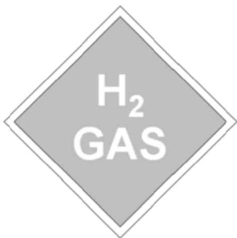
Picture 6.5-3 Marking for identification of a gaseous hydrogen powered car. Colours: green background, white border and white letters (border and letter, or background, shall be retro-reflective)
