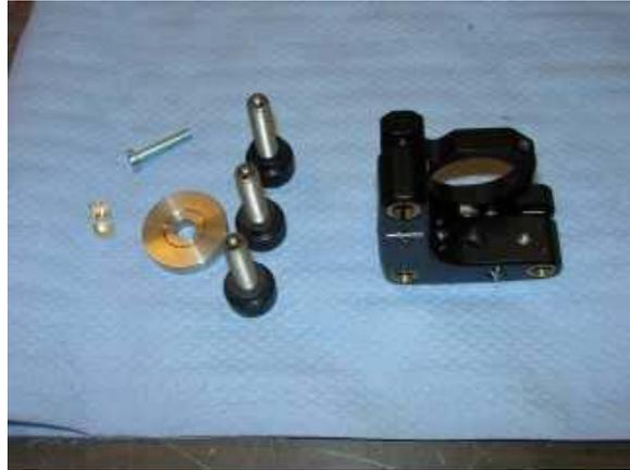
Figure 1: Photo of disassembled mirror mounts.
