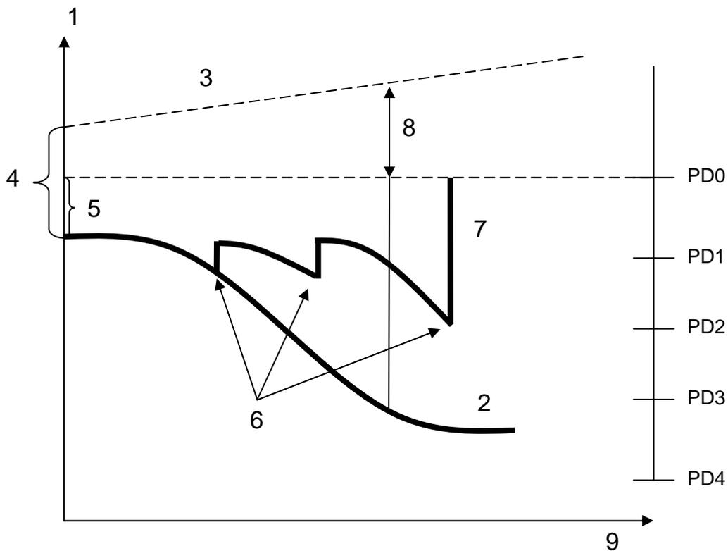
Figure 2. The building performance cycle with performance degrees PD (adapted from ISO 15686-7). The upper (jagged) curve represents the performance for a building, a part thereof, or a component where an acceptable performance is regained with regular maintenance and ultimately by replacement.
