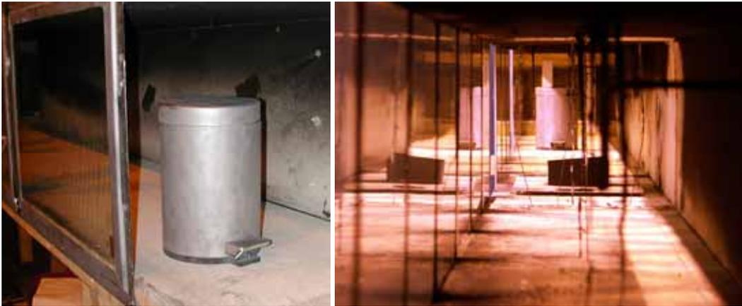
**Figure 4.2** The target consisted of a blasted aluminium bucket. This was placed 2– 2.5 m into the tunnel (the distance was varied between the tests), i.e. 7.5–8 m from the exit from the tunnel. The pool with heptane was placed 5 m from the exit of the tunnel. The photos are from Test 6.
