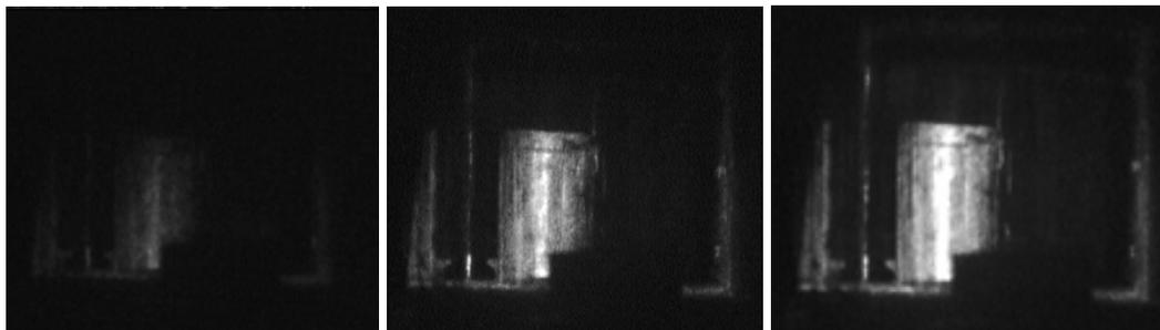
**Figure 5.6** Series of images from the Aqua Lynx system. From left to right, the smoke gets thinner during the last 30 s of the fire.
