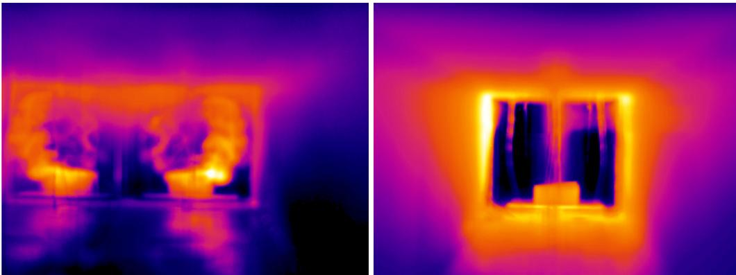
**Figure 5.13** Images from the ThermaCam® SC2000. The left image is taken 2 minutes after ignition, while the right image is taken a few minutes after the fire.
