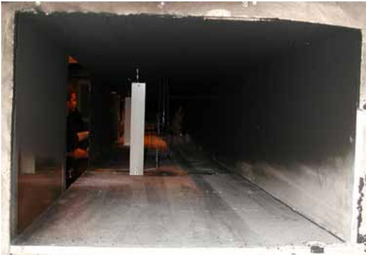
**Figure 4.3** White target plates were used in Test 9, to get a good picture of the distance the different systems could “see” through the smoke.
