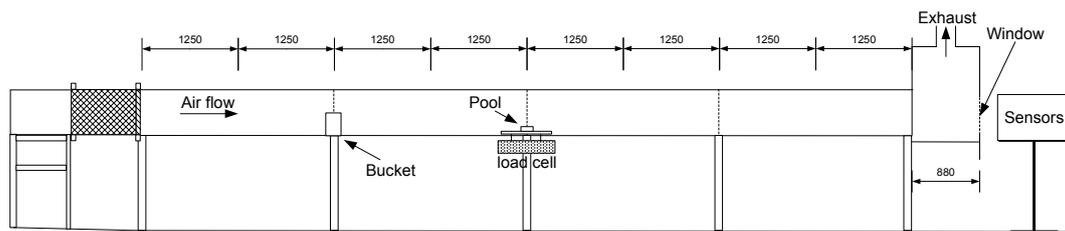
Figure 2.1 Side view of the model-scale tunnel.
