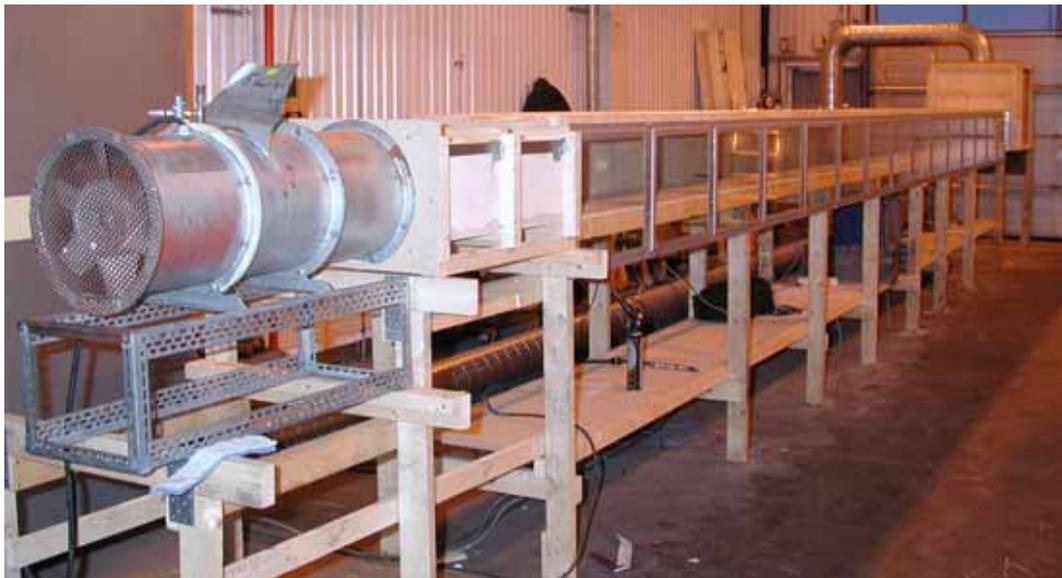
Figure 2.2 The model-scale tunnel built at SP Fire Technology.
