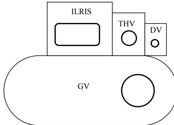
**Figure 3.1** A package of optical sensors including a gated viewing camera (GV), a laser scanner (ILRIS), a thermovision camera (THV), and a DV camera.
