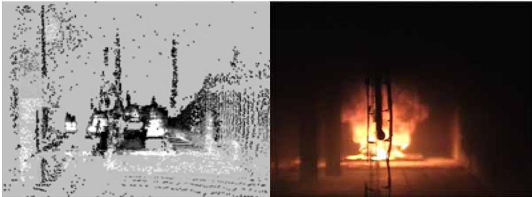
Figure 5.9 Results from ILRIS-3D and photo from Test 9, 3 minutes after ignition.
