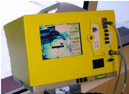
**Figure 3.3** The laser scanner Optech ILRIS-3D**Table 3.2** Technical data of Optech ILRIS-3D
