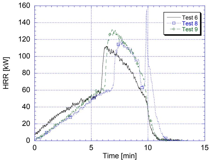
Figure 5.1 Heat release rate (HRR) for the three tests (Test 6, Test 8 and Test 9).
