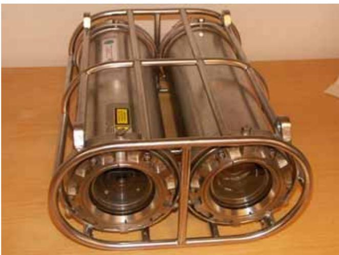
**Figure 3.2** The gated viewing laser system Aqua Lynx.
