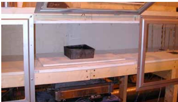
**Figure 4.1** The heptane pool on a Promatect®-H board, connected to a load cell.
