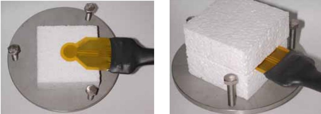
**Figure 3.** TPS sensor is clamped between two samples of material. Note that the material in the photo is not part of this study but is only used to illustrate the method.
