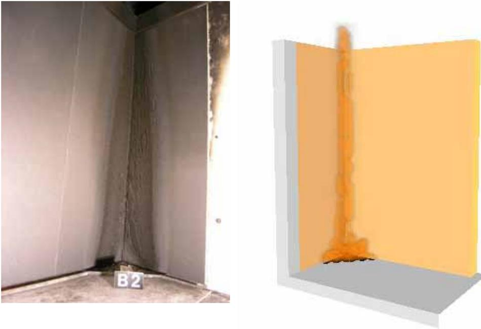
**Figure 23.** Area of the panels involved in the fire, flames in FDS model compared to photo after the test. The dark area in the left photo is the expanded INCA material at the end of the test. The geometry of model is reversed compare to the test set-up.
