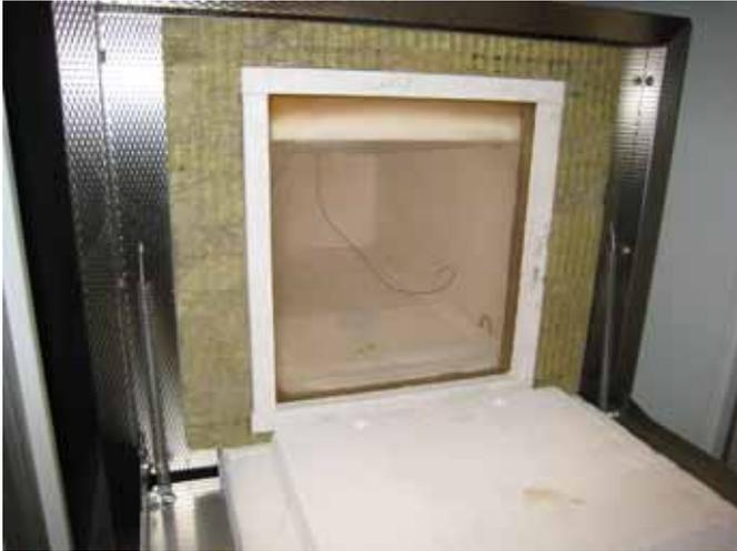
**Figure 1.** Furnace and the pane of fireproof glass
