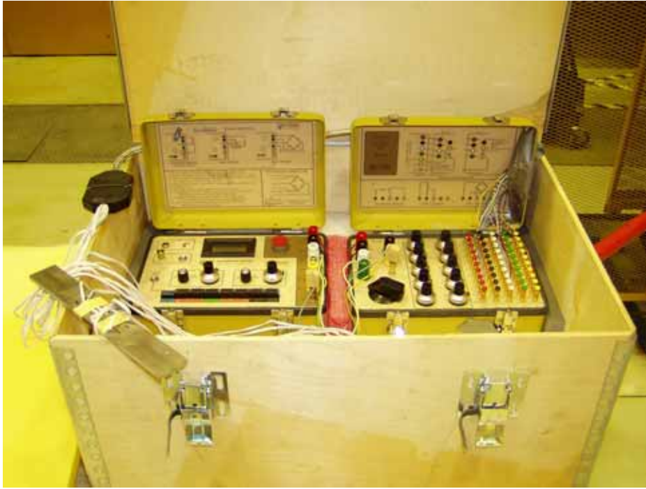
Figure 5. The strain measuring system
