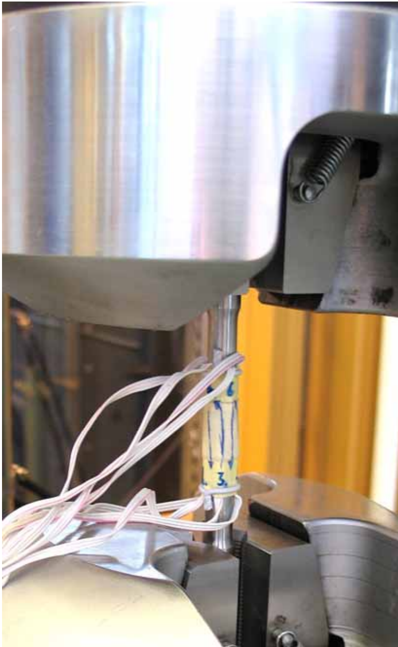
Figure 4. Round test specimen mounted in hydraulic grips in one of the participant's testing machines.
