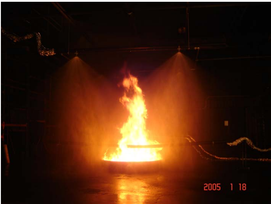
Photo 2 Fire control of the 3,5 MW diesel pool fire using the water discharge density of 5,0 mm/min.
