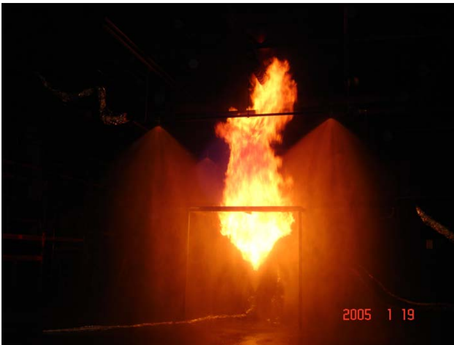
Photo 4 The 3,5 MW diesel spray fire at the 5,0 mm/min water discharge density.
