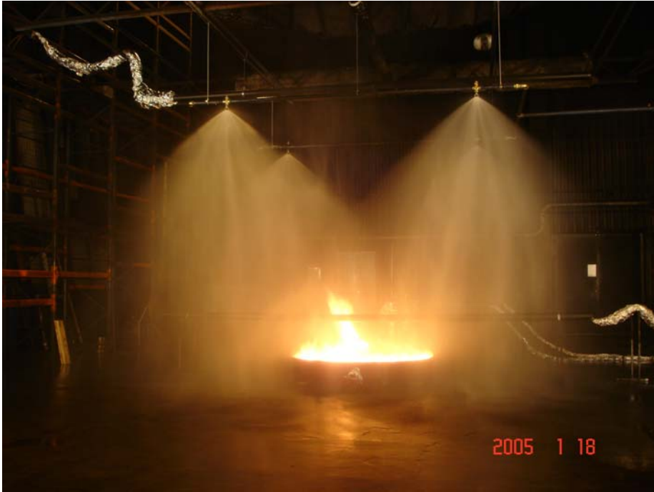
Photo 3 Fire suppression of the 3,5 MW diesel pool fire using the water discharge density of 7,5 mm/min.
