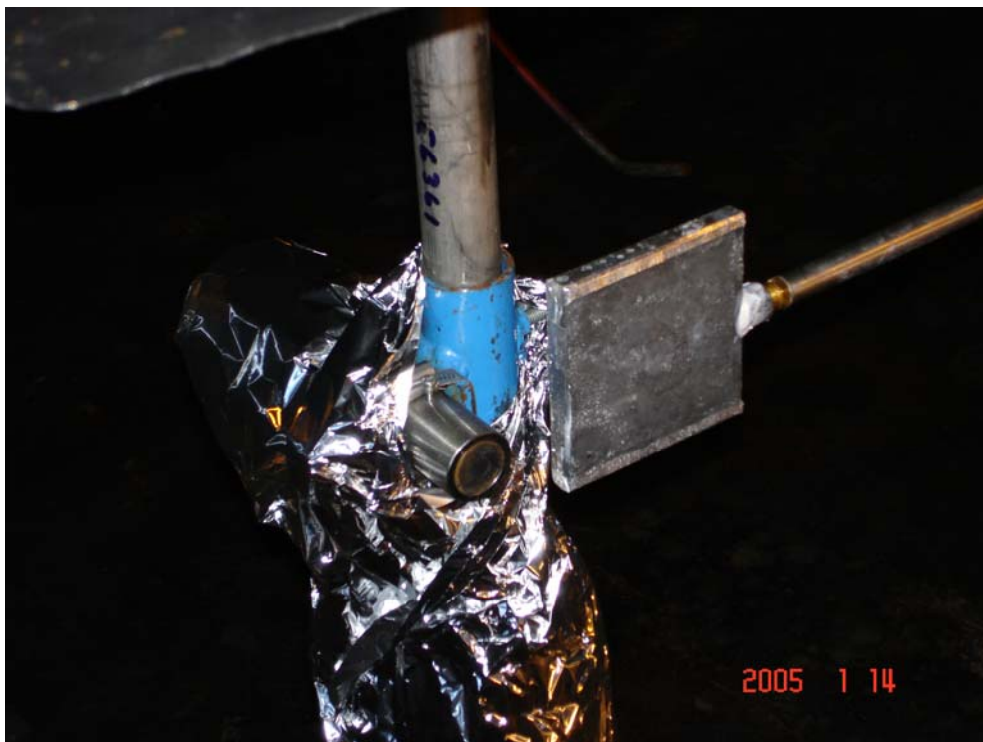
Figure 4 One of the heat flux meters and the adjacent Plate Thermometer.
