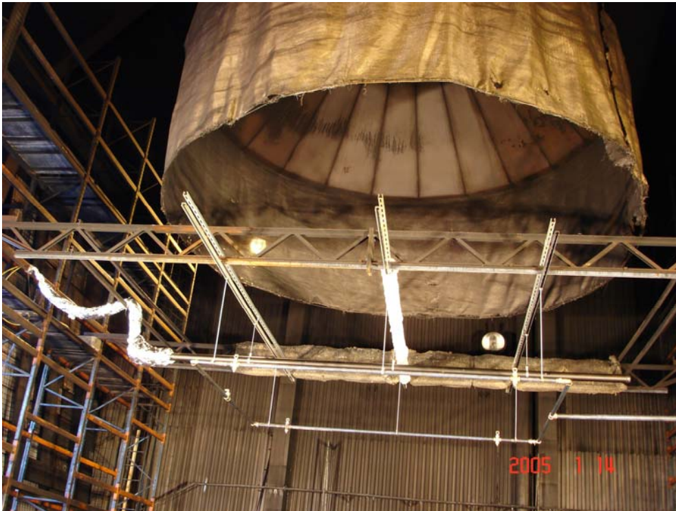
Figure 3 The Industry Calorimeter was used to measure the Heat Release Rates from the fires. The system pipe-work and the uppermost Pipe Thermometer can be seen below the calorimeter.
