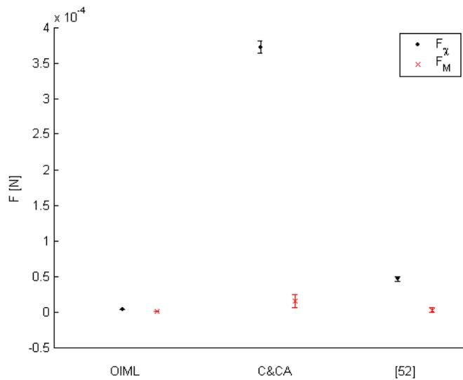
Figure D.1. Measured forces for the 1 kg mass standards used in the international comparison.
