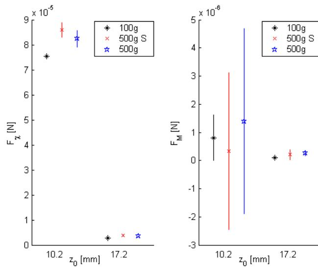
Figure D.3. Forces measured when the mass standards are placed with the envelope surface on the susceptometer bridge.
