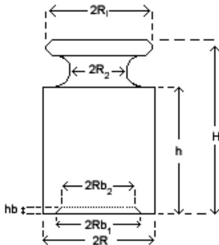
Figure E.1. The dimensions of an OIML mass standard.
