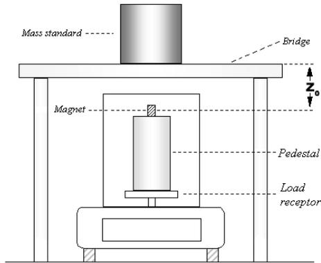
Figure 4. Design of a susceptometer.
