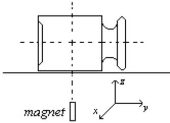
Figure 16. The axis is of the magnet is perpendicular to the principal axis of the mass standard.
