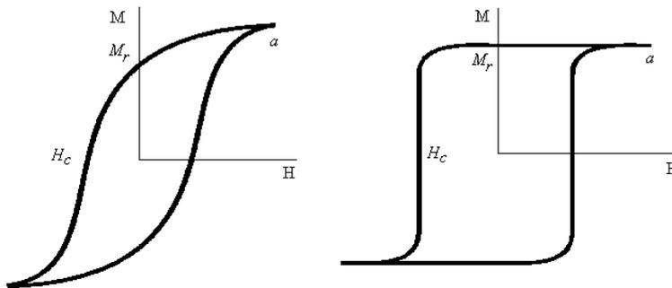
Figure 2. Hysteresis curves for soft alloys (left side) and for hard alloys (right side).
