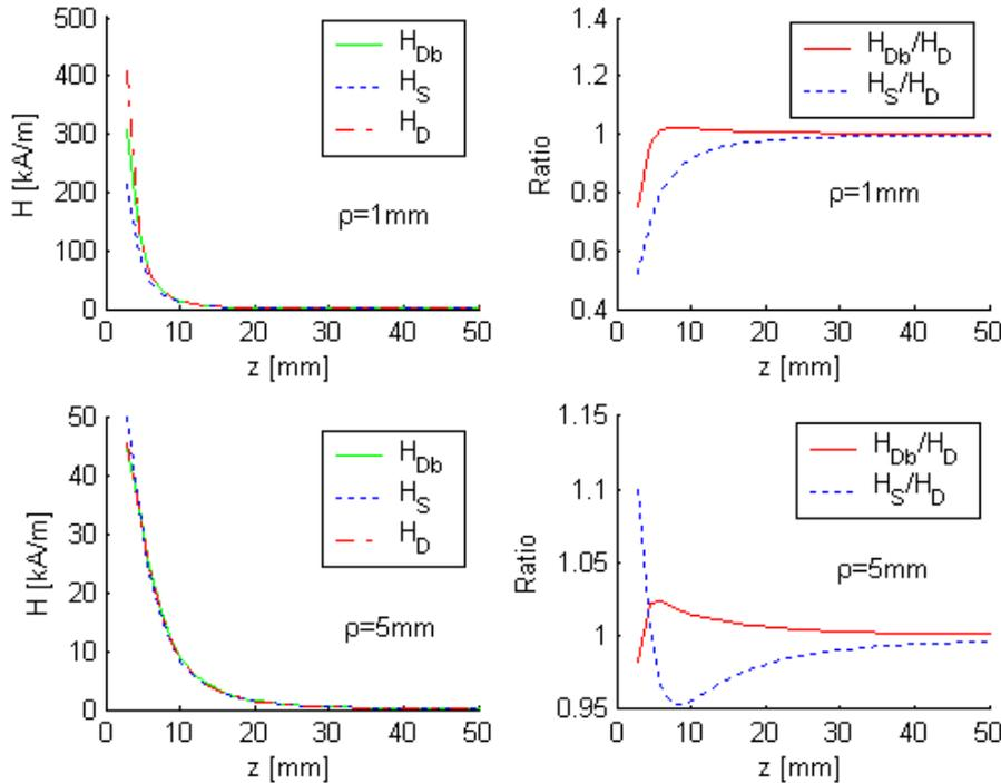
Figure 8. The magnitudes of magnetic field intensities calculated at  $\rho = 1$  mm and  $\rho = 5$  mm.
