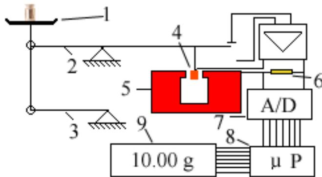
Figure 3. A schematic diagram of a laboratory balance with electromagnetic force compensation.
