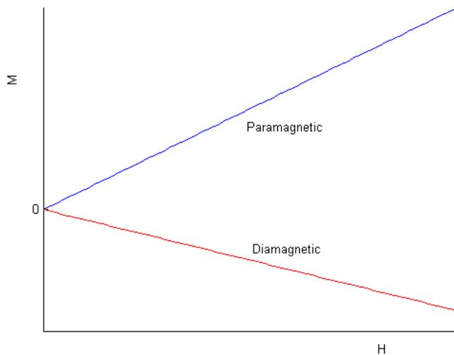
Figure 1. Magnetization due to external  $H$ -field for diamagnetic and paramagnetic materials.
