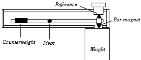
Figure 6. The design of a permeability indicator.
