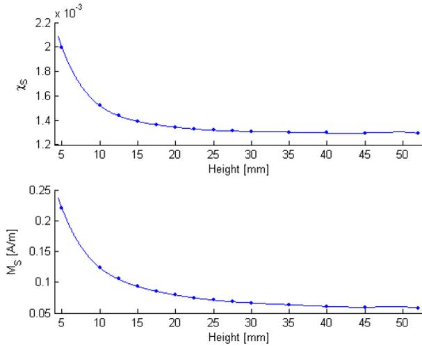
Figure 14. Susceptibility and permanent magnetization of 1 kg cylindrical mass standard calculated at different heights (dots).
