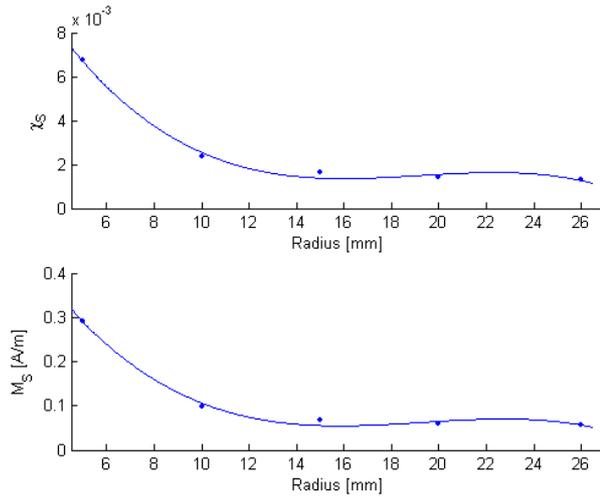
Figure 15. Susceptibility and permanent magnetization calculated at various radii (dots).
