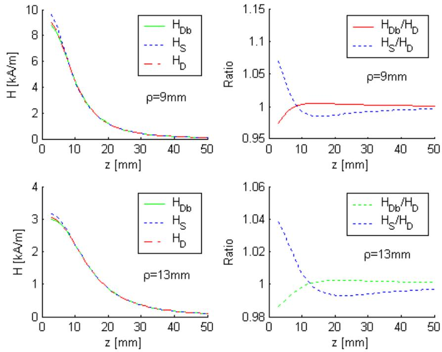
Figure 9. The magnitudes of magnetic field intensities calculated at  $\rho=9\text{ mm}$  and  $\rho=13\text{ mm}$ .
