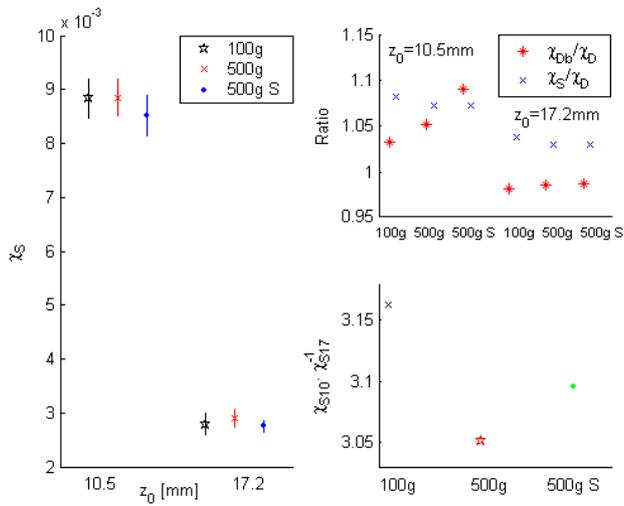
Figure 17. Susceptibilities calculated at  $z_0 = 10.5$  mm and  $z_0 = 17.2$  mm and ratio of susceptibilities.
