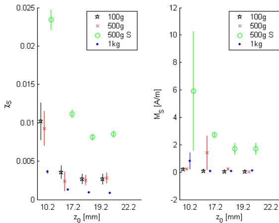
Figure 13. Susceptibility and permanent magnetization calculated at different distances  $z_0$ .
