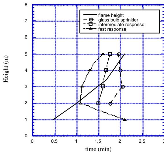
Figure 1 Typical sprinkler response to a fire ignited in the vertical flue (based on information given in reference [10]).
