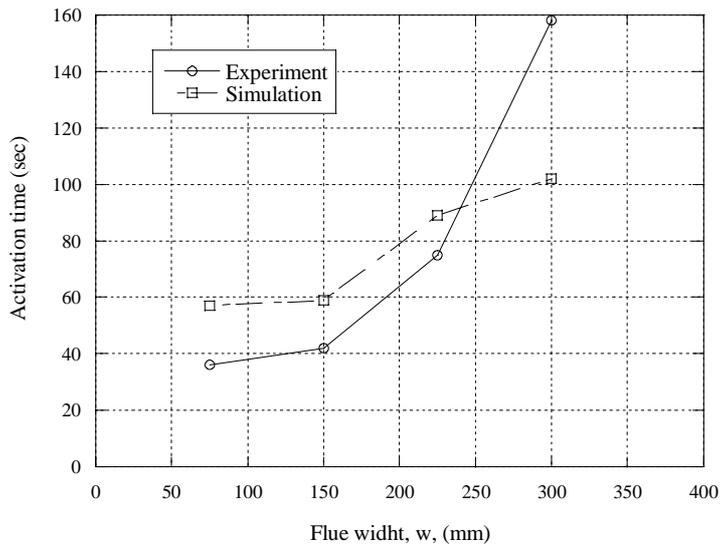
Figure 15 Comparison between measured and simulated activation time of in-rack sprinkler at  $z=4.87$  m.
