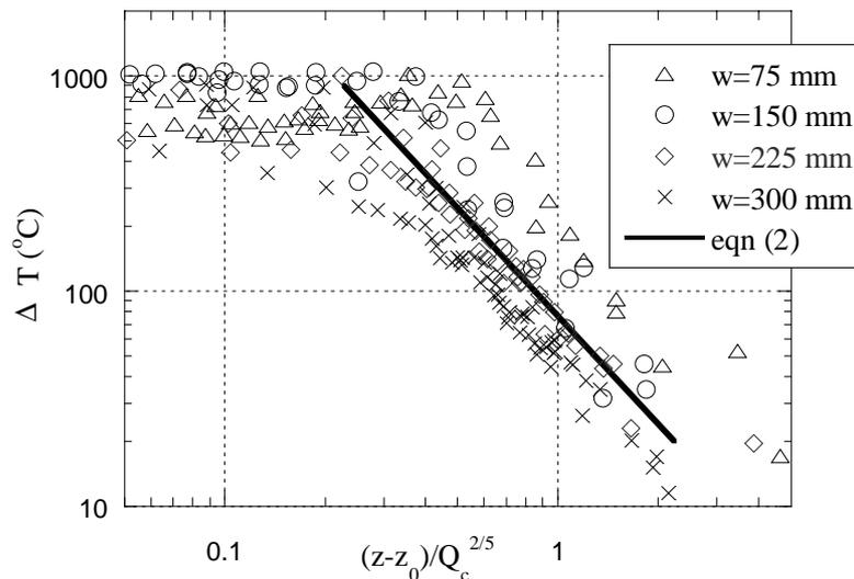
Figure 6 The excess centreline temperature versus  $(z-z_0)/Q_c^{2/5}$  for different flue widths,  $w$ . The temperatures were measured at tiers two, three and four. The solid line is equation (2). Equation (3) was used to calculate  $z_0$ .
