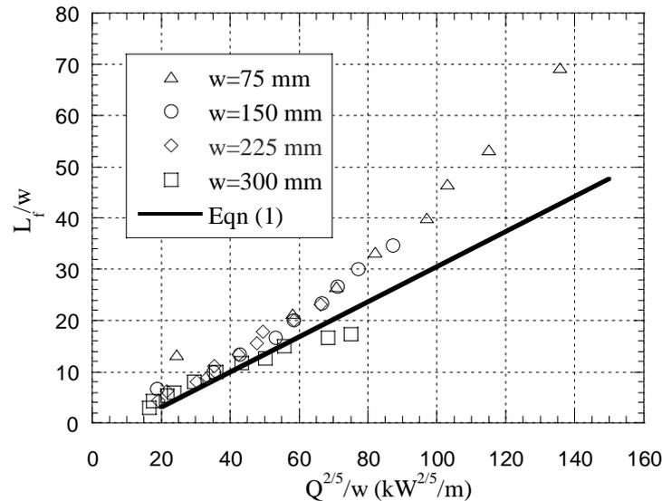
Figure 5 The non-dimensional flame height ( $L_f/w$ ) plotted as a function of  $Q^{2/5}/w$  for the large-scale tests. Equation (1) is based on earlier tests using model scale tests and one large-scale test.  $W$  is the flue width.
