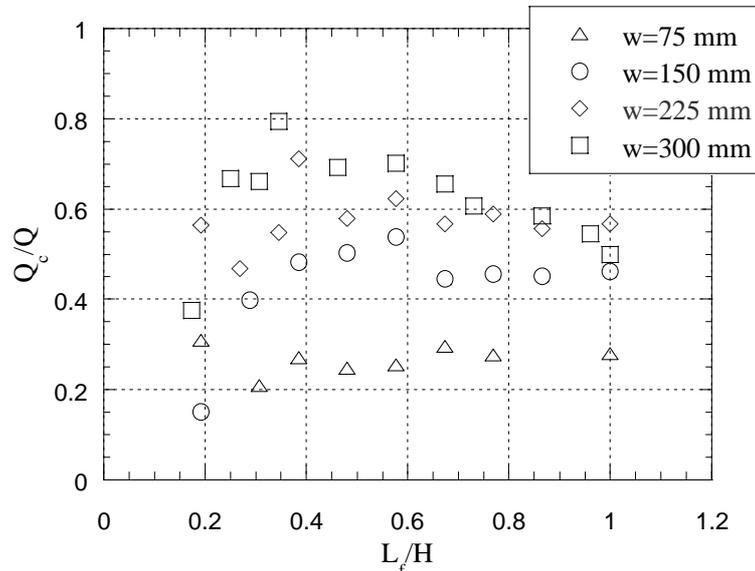
Figure 13 The ratio  $Q_c/Q$  plotted as a function of  $L_f/H$  for different flue widths.
