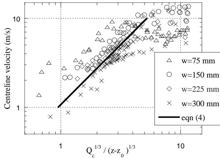
Figure 8 The in-rack centreline velocity as a function of  $Q_c^{1/3} / (z - z_0)^{1/3}$  for the four different flue widths,  $w$ , and tiers two to four.
