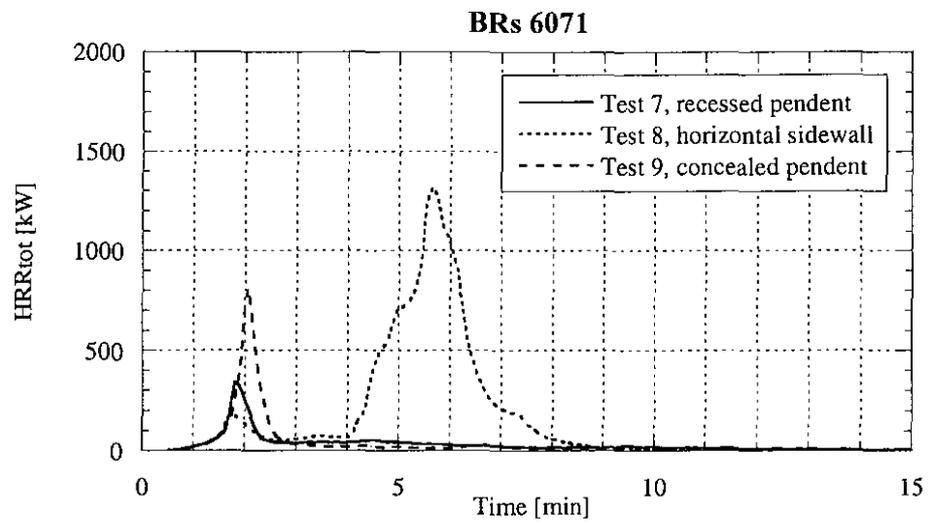
Figure 4 *Total heat release rate histories for the sprinkler tests where ignition took place at the seat, close to the bottom of the backrest of the chair.*
