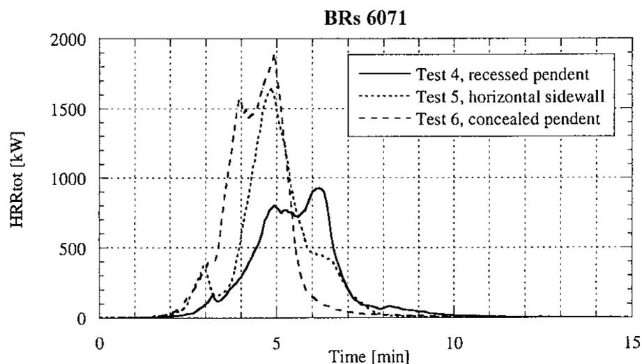
Figure 3 Total heat release rate histories for the sprinkler tests where ignition took place at the bottom, left hand side of the upholstered chair.
