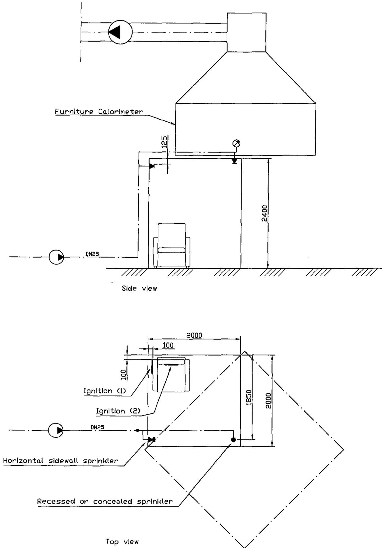
Figure 1 The test set-up showing the Furniture Calorimeter that was used to determine the heat release rate of the fires.
