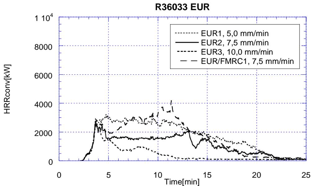
*Figure 4* Convective heat release rate histories for the EUR Standard Plastic commodity tests and for the test with EUR Standard Plastic commodity cartons with FMRC plastic cups. Ignition at 02:00, manual extinguishment, if any, at 24:00.
