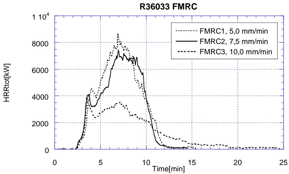
Figure 1 Total heat release rate histories for the FMRC Standard Plastic commodity tests. Ignition at 02:00, manual extinguishment, if any, at 24:00
