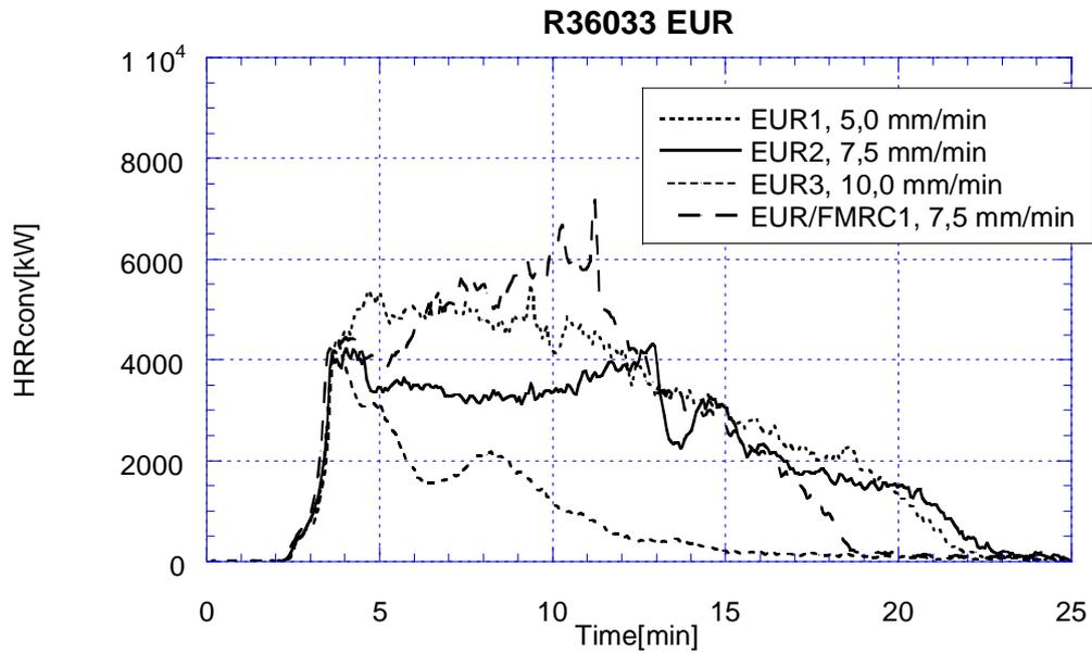
*Figure 3* Total heat release rate histories for the EUR Standard Plastic commodity tests and for the test with EUR Standard Plastic commodity cartons with FMRC plastic cups. Ignition at 02:00, manual extinguishment, if any, at 24:00.
