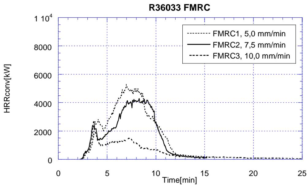
Figure 2 Convective heat release rate histories for the FMRC Standard Plastic commodity tests. Ignition at 02:00, manual extinguishment, if any, at 24:00.
