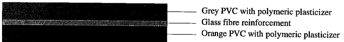
Figure 2: Composition of "Protan GO"
