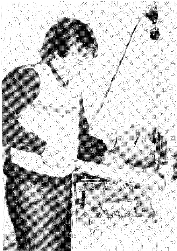
Fig. 5. The straw samples for EMC trials were prepared by cutting into suitable pieces. Photo G. Lundin.
