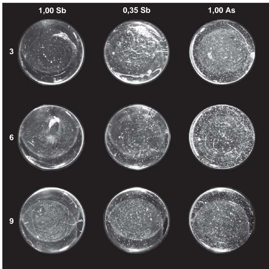
**Figure 4** The variation in bubbles for pieces with varying amount nitrate, 3, 6 or 9 kg added NaNO<sub>3</sub> per 100 kg sand, and different fractions of antimony, 1,00 Sb(III), 0,35 Sb(III) or 1,00 As(III). The bubbles show up as light spots.
