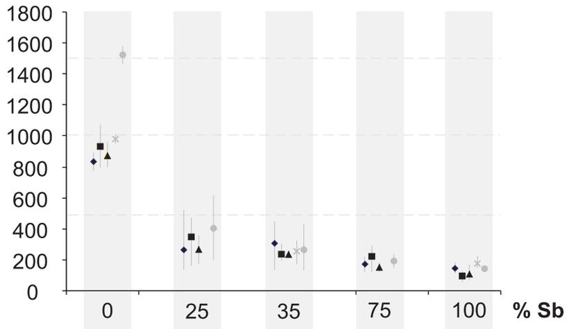
**Figure 3** Simplification of figure 2. The mean value of the number of bubbles found is plotted for the different fractions of added Sb and the error bars shows the variation in the number of bubbles. The addition are represented by  $\diamond$  for 3 kg  $\text{NaNO}_3$ ,  $\square$  for 6 kg  $\text{NaNO}_3$ ,  $\triangle$  for 9 kg  $\text{NaNO}_3$ ,  $\times$  for 11 kg  $\text{KNO}_3$  for refining with Sb(III)/As(III) and  $\bullet$  for refining with Sb(V)/As(V).
