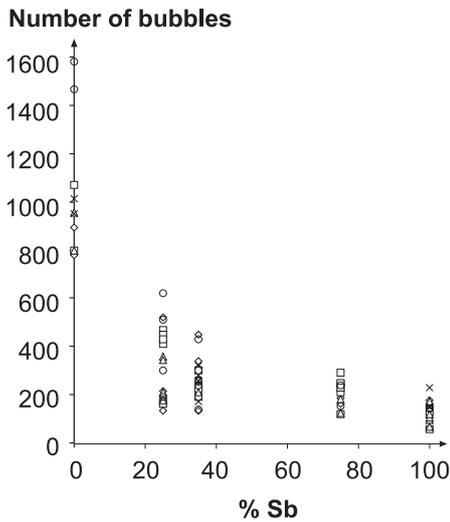
**Figure 2** Number of bubbles as a function of the antimony content, see table 1. The Sb(III)/As(III) series are represented with diamonds ( $\diamond$ ) when 3 kg of  $\text{NaNO}_3$  are added, with squares ( $\square$ ) for 6 kg  $\text{NaNO}_3$ , with triangles ( $\triangle$ ) for 9 kg  $\text{NaNO}_3$ , while the cross ( $\times$ ) is with addition of 11 kg  $\text{KNO}_3$  and the circles ( $\bullet$ ) are for the Sb(V)/As(V) system. All amounts are additions per 100 kg sand.
