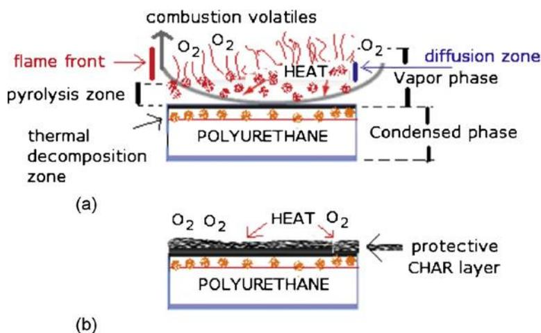
Figure 5. Typical process taking place during the combustion of PU in the absence (a) and presence (b) of an intumescent flame retardant.
