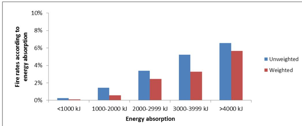
Figure 4: Fire rates in crashes according to energy absorption. CDS data, 2005-2014, unweighted and weighted. Note: up to 30% had a fire entry “unknown”, and of the ones who had a fire, 50 to 60% had an unknown energy adsorption.
