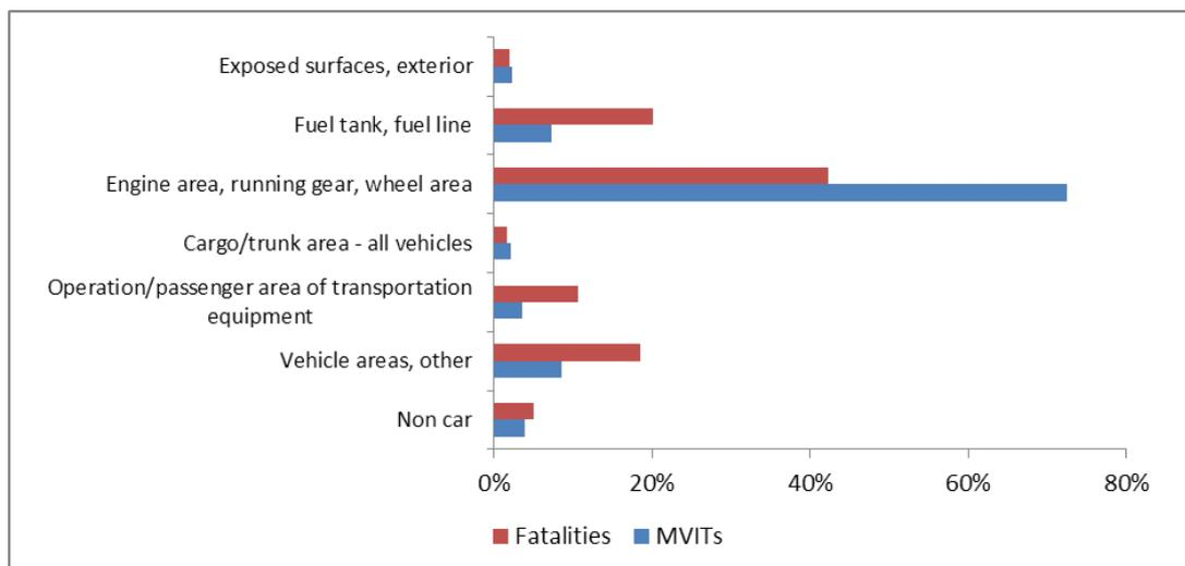
**Figure 3. Area of fire origin for all MVITs fire cases and for all fatalities, when collision is the primary factor of ignition. NFIRS data, 2005-2013. Unknowns (8 to 15%) are apportioned.**
