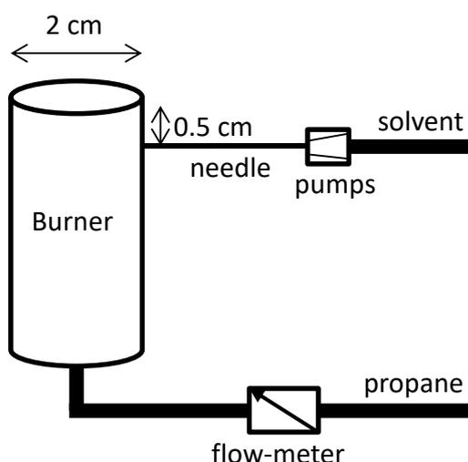
**Figure 12. Schematic illustration of burner**
