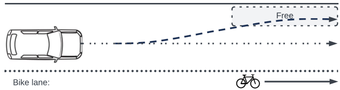
Fig. 2. A car approaches a bicycle with an area that is classified as free. Strategies for passing the bicycle in this situation include driving straight ahead (dotted arrow) or swerving to the left in the lane (dashed arrow). The figure also illustrates that selecting either path over the other constitutes a risk transfer between road users present in the situation, including undetected road users due to the inherent uncertainties in perception, but no statistical risk transfer.
