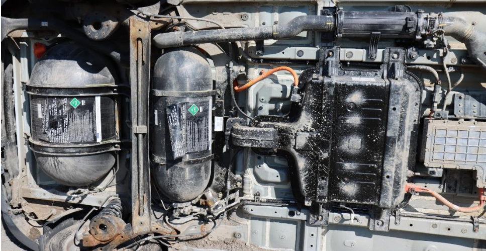
Figure 2 Hydrogen vehicle with two Type IV composite tanks placed at the rear end of the vehicle.
