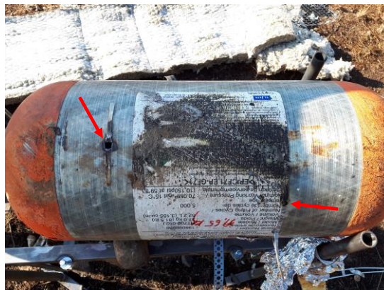
Fig. 9. Two successful penetrations at first shot; one big hole to the left (#5b that resulted in a large jet flame) and a small to the right (#5a that resulted in minor leakage). (Photo: RISE)
