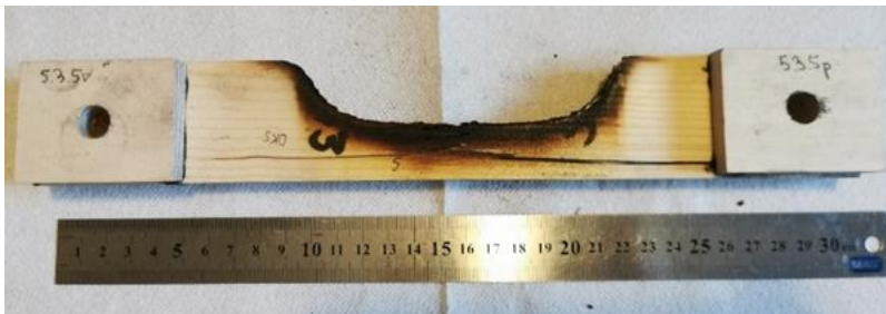
Figure 10. Test series 2 specimen after cleaning.
