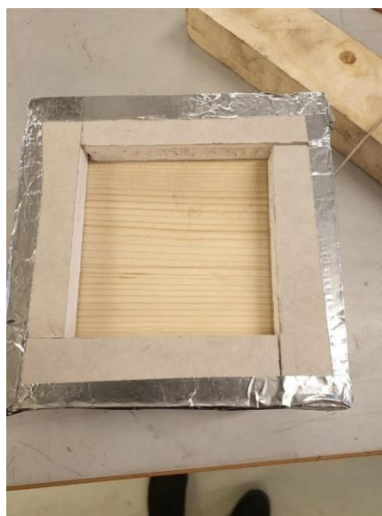
Figure 17. Specimen protected with plasterboard and aluminium tap.
