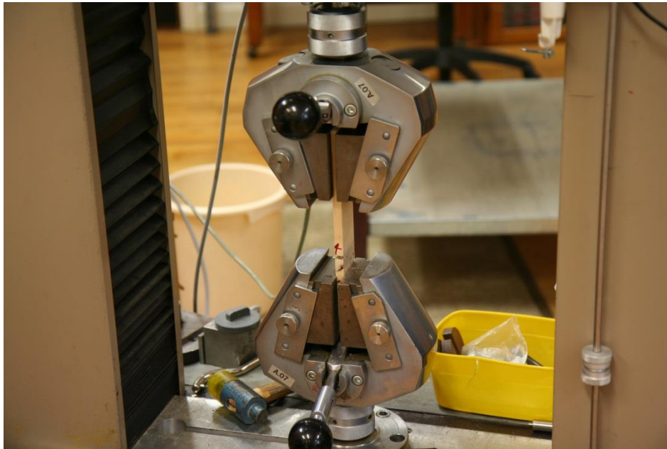
Figure 4. Tension test at ambient temperature.
