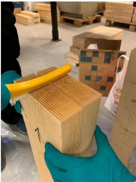
Figure 1. Manual application of adhesive on finger joint.
