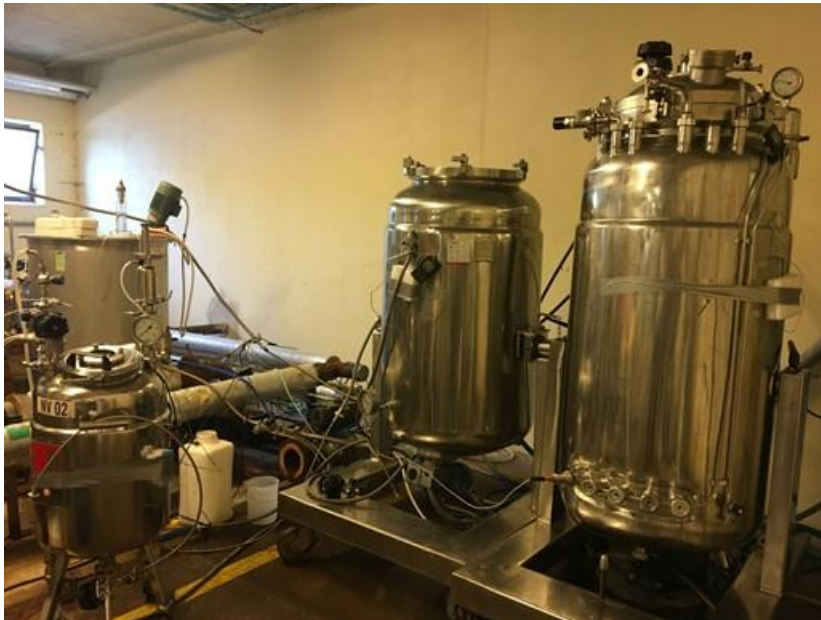
Pilot-scale reactors at Anneberg. The larger one is of the 430 L working volume.
