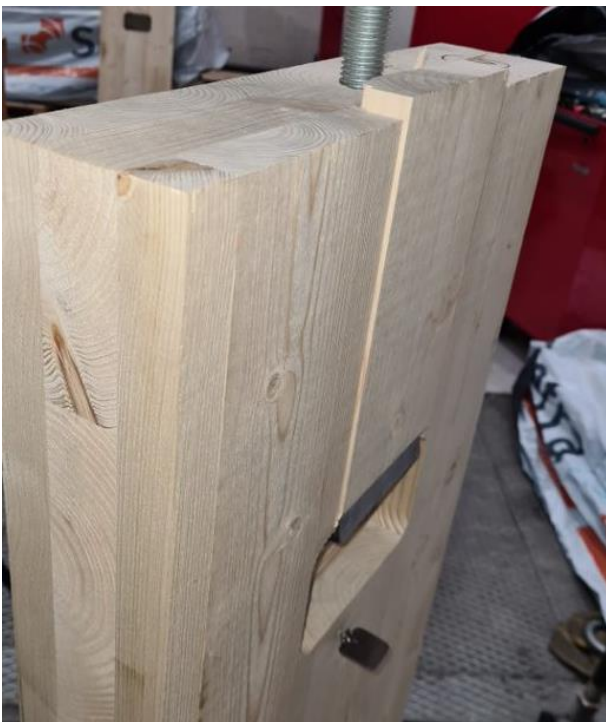
Figure 13: Test 2 shear failure of outer layer
