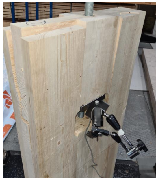
Figure 10: Test 1 shear failure
