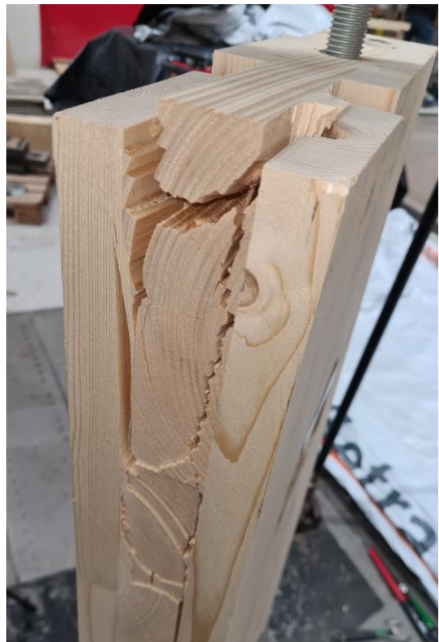
Figure 15: Test 3 failure in middle layer
