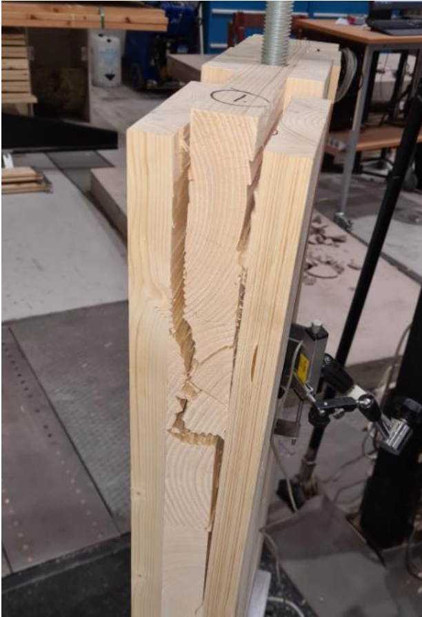
Figure 12: Test 1 rolling shear failure in mid-layer
