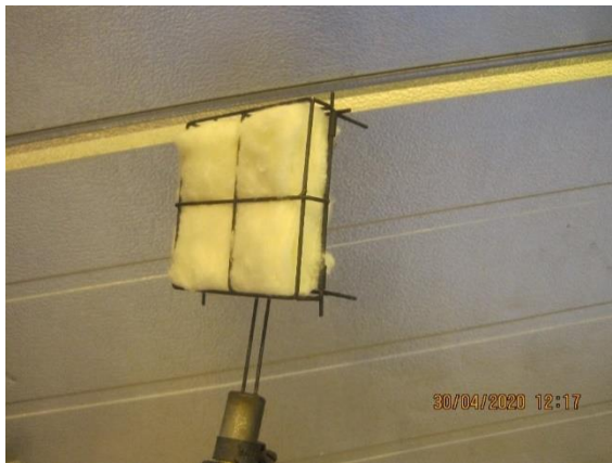
Figure 1. Cotton-wool pad used for testing ignition (flaming or glowing) on the unexposed side. Size: 100*100*20 mm. 3-4 g of cotton
