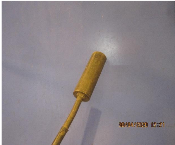
Figure 2. Gap gauges for measuring openings in tested specimen. 25 mm in diameter
