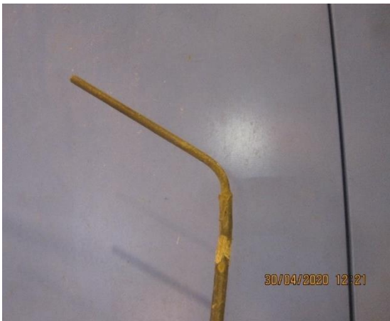
Figure 3. Gap gauges for measuring cracks in tested specimen. 6 mm in diameter to move 150 mm in different directions of the crack.
